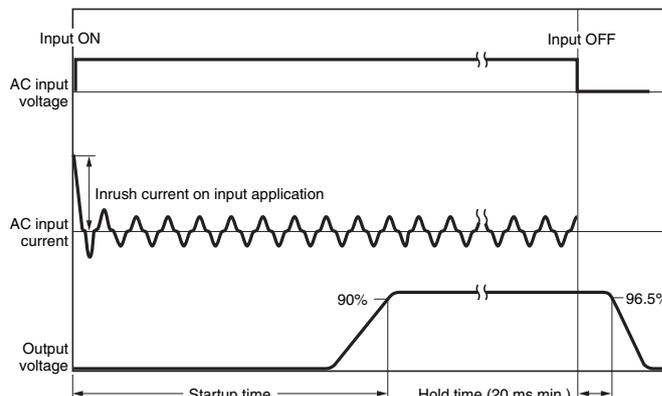
**Note:** A maximum startup time of 1,000 ms is required. Construct a system configuration that considers the startup time of other devices.
