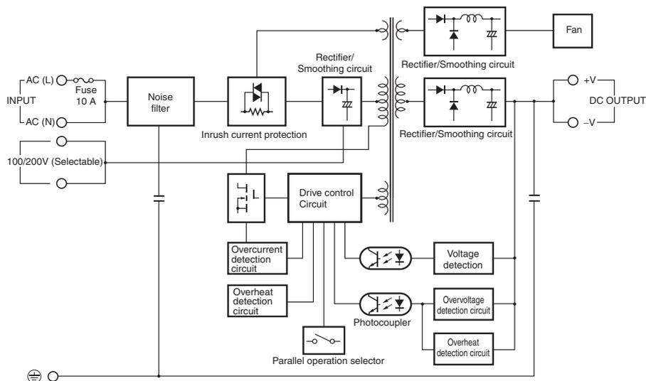
Note: Short-circuit the input voltage selector terminals if the input is 100 to 120 VAC. Keep the terminals open if the input is 200 to 240 VAC.
