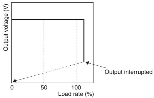
If an excessive current flows for 5 s or more, the output will be turned OFF and simultaneously the protection-ON alarm indicator will be lit. To reset the S8JX, turn OFF the power, leave the S8JX for at least three minutes, and then turn it ON again.
