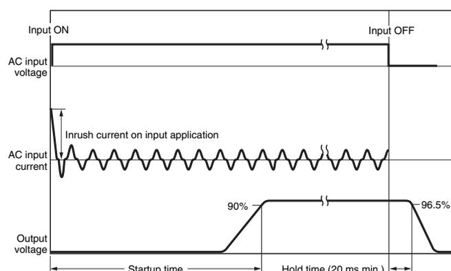
**Note:** A maximum startup time of 500 ms is required (650 ms for 300 W). Construct a system configuration that considers the startup time of other devices.
