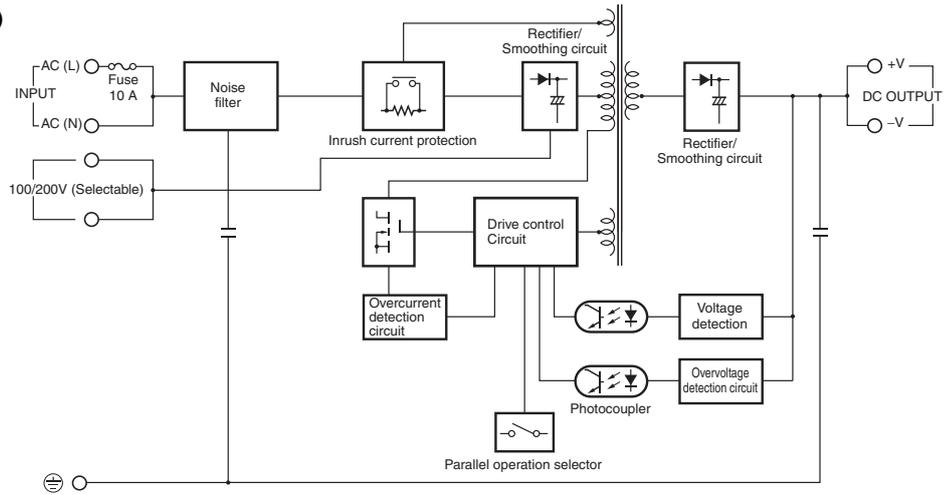
**Note:** Short-circuit the input voltage selector terminals if the input is 100 to 120 VAC.
