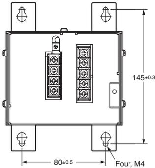
**Attaching the Mounting Brackets**
