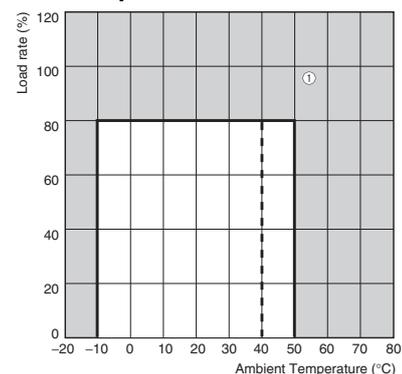
— Solid line Front-mounting, Bottom-mounting, DIN Rail mounting, Side mounting (300W 5V, 12V/ 600W 24V, 48V Models)
