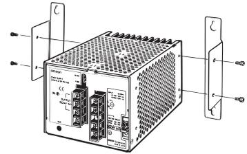
**Note:** To provide ventilation space, the body will shift forward by 21.6 mm from the mounting surface.
