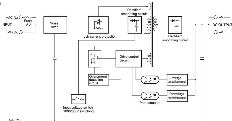
Note: Set the input voltage switch to "115V" for 100 to 120 VAC and to "230V" for 200 to 240 VAC.
