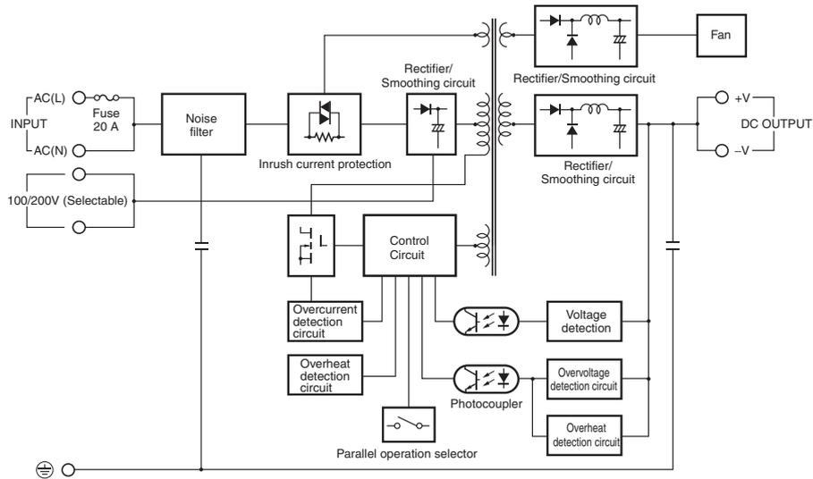
**Note:** Short-circuit the input voltage selector terminals if the input is 100 to 120 VAC.
