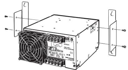
**Note:** To provide ventilation space, the body will shift forward by 23.6 mm from the mounting surface.
