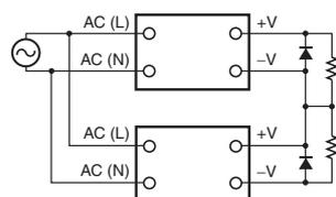
**Note: 1.** If the load is short-circuited, a reverse voltage will be generated inside the Power Supply. If this occurs the Power Supply may possibly deteriorate or be damaged. Always connect a diode as shown in the figure. Select a diode having the following ratings.
