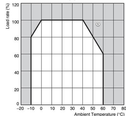
**Note: 1.** Internal parts may occasionally deteriorate or be damaged. Do not use the Power Supply in areas outside the derating curve (i.e., the area shown by shading ① in the above graph).
