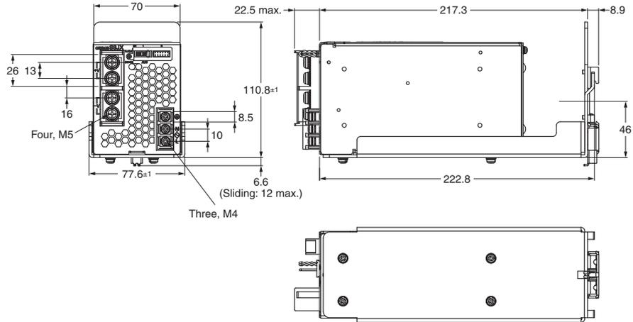
**Note:** Use a metal DIN Rail when mounting a 300-W model to a DIN Rail.
