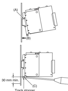
To dismount the Power Supply, pull down portion (C) with a flat-blade screwdriver and pull out the Power Supply.
