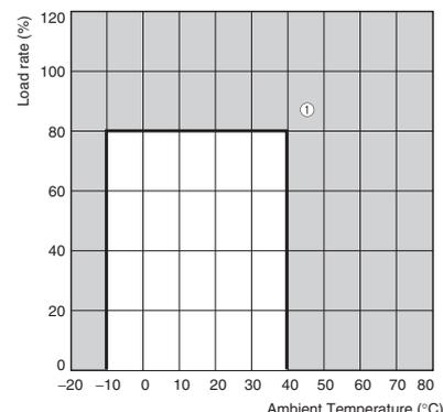
**Note: 1.** Internal parts may occasionally deteriorate or be damaged. Do not use the Power Supply in areas outside the derating curve (i.e., the area shown by shading ① in the above graph).
