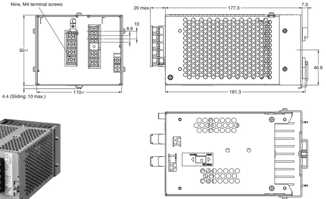
**Note:** Use a metal DIN Rail when mounting a 300-W model to a DIN Rail.
