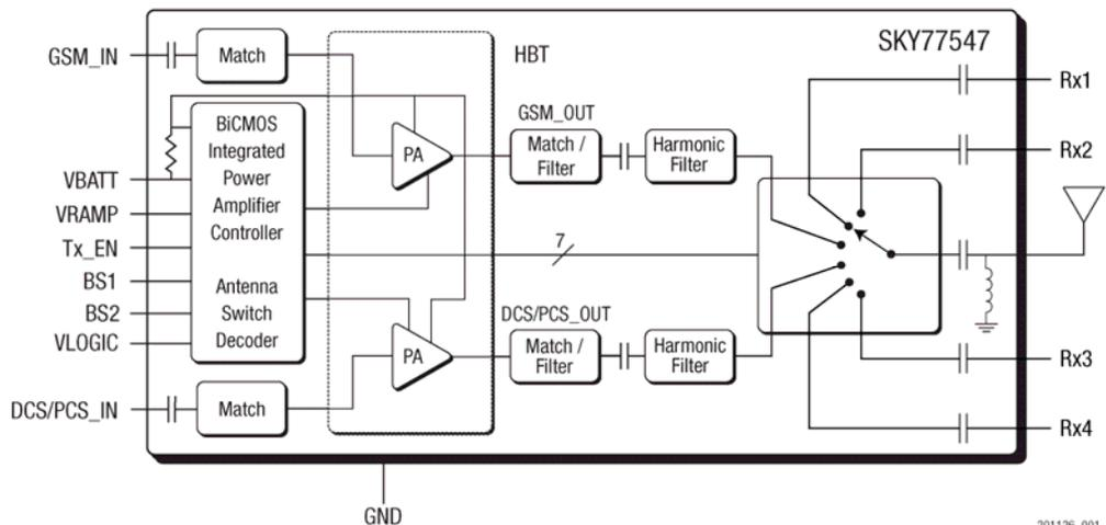
Figure 1. SKY77547 Functional Block Diagram
