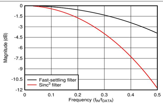
Figure 8-5. Fast-Settling and Sinc<sup>3</sup> Digital Filter Response, Pass-Band Detail
