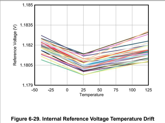
**Figure 6-29. Internal Reference Voltage Temperature Drift**
