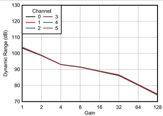
Figure 6-21. Dynamic Range vs Gain Across Channels
