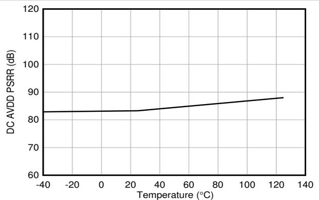
**Figure 6-15. DC AVDD PSRR vs Temperature**
