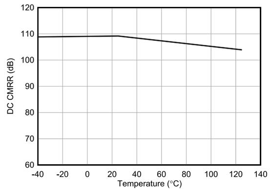
**Figure 6-13. DC CMRR vs Temperature**
