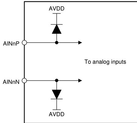
**Figure 8-1. Input ESD Protection Circuitry**
