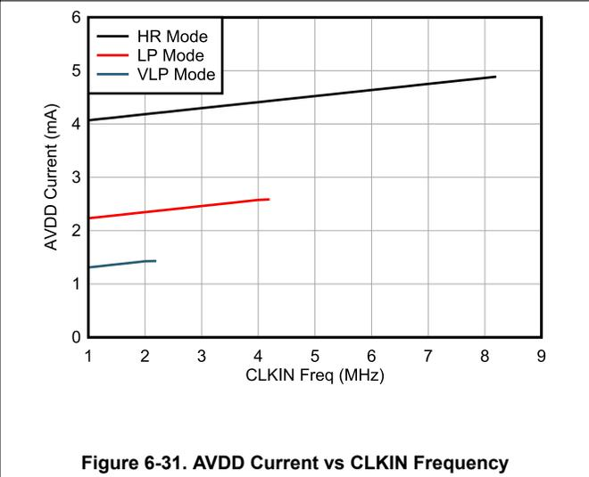
**Figure 6-31. AVDD Current vs CLKIN Frequency**
