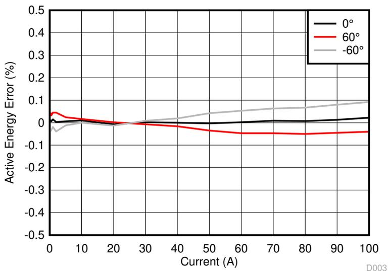
**Figure 9-8. Cumulative Phase Active Energy % Error Versus Current**
