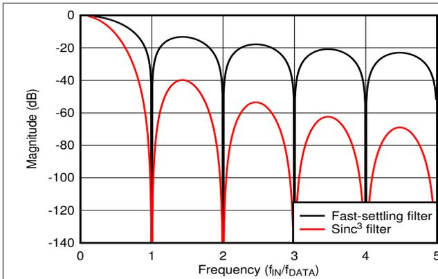
Figure 8-4. Fast-Settling and Sinc<sup>3</sup> Digital Filter Response
