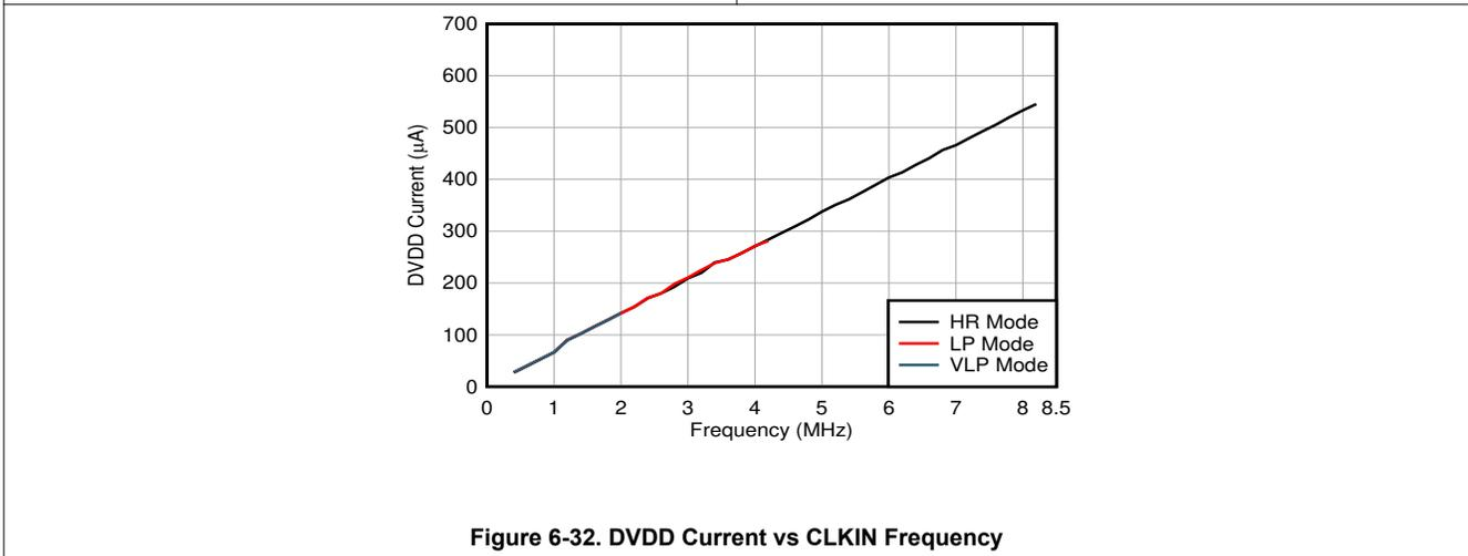
**Figure 6-32. DVDD Current vs CLKIN Frequency**
