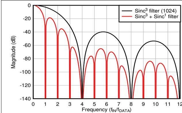
Figure 8-6. Digital Filter Response for OSR = 1024 and OSR = 4096
