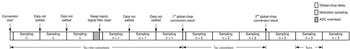
Figure 8-16. Conversion Timing With Global-Chop Mode Enabled
