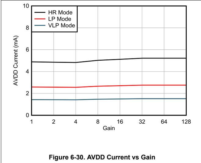
**Figure 6-30. AVDD Current vs Gain**
