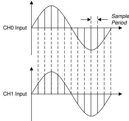
**Figure 8-9. Two Channel Outputs With Equal Phase Settings**
