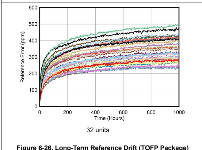
Figure 6-26. Long-Term Reference Drift (TQFP Package)
