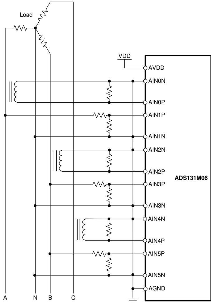
**Figure 9-3. Three-Phase Current and Voltage Measurement Front-End**
