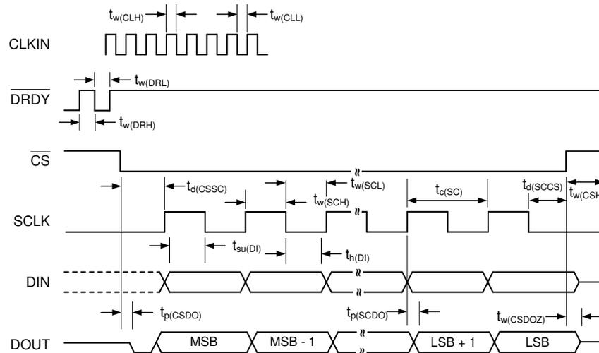
SPI settings are CPOL = 0 and CPHA = 1.  $\overline{CS}$  transitions must take place when SCLK is low.
