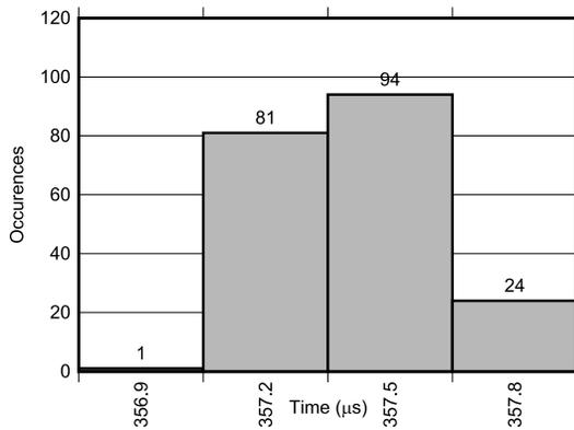
Figure 6-6. Startup Time Histogram
