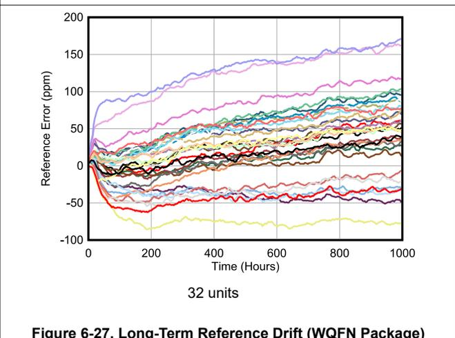
Figure 6-27. Long-Term Reference Drift (WQFN Package)
