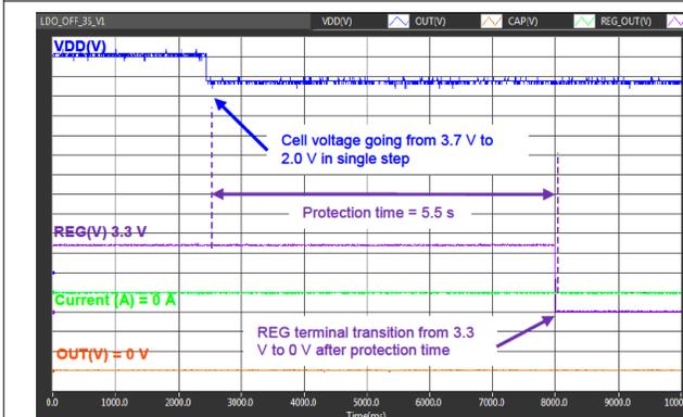
Figure 9-6. Undervoltage Detection to Turn Off the Regulator
