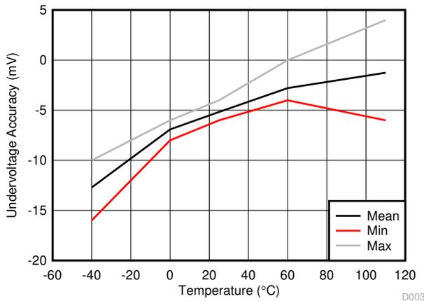
**Figure 7-3. Undervoltage Accuracy**
