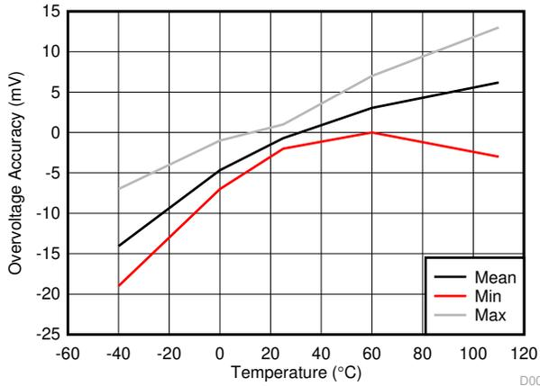
**Figure 7-1. Overvoltage Threshold ( $V_{OV}$ ) vs. Temperature**
