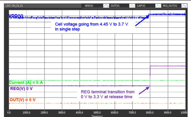
Figure 9-7. Undervoltage Release to Switch On the Regulator
