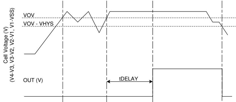
Figure 8-1. Timing for Overvoltage Sensing for OUT
