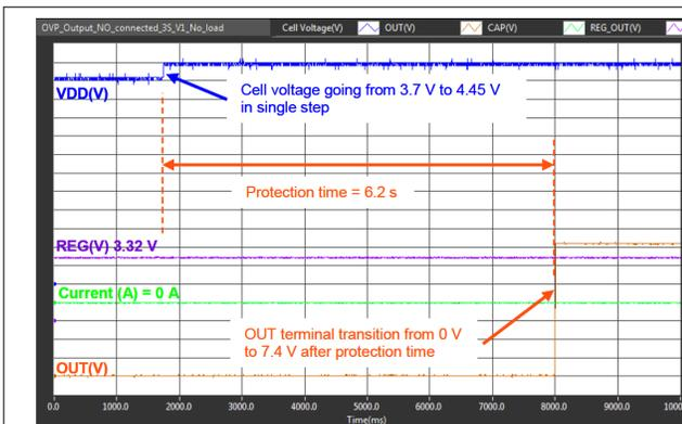
Figure 9-4. Overvoltage Protection
