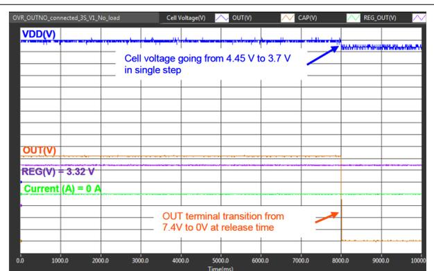
Figure 9-5. Overvoltage Protection Release
