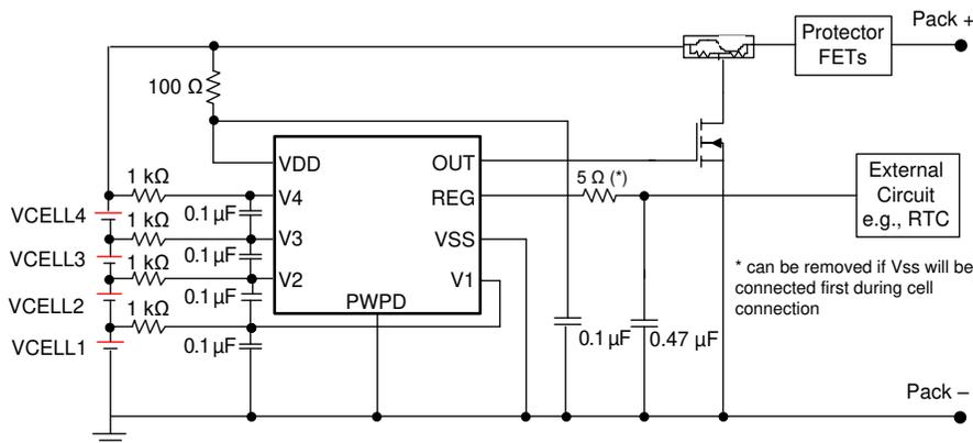
Figure 9-1. Application Schematic
