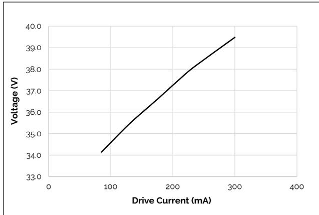
**Figure 2: V4B HD Drive Current vs. Voltage ( $T_j = T_c = 25^\circ\text{C}$ )<sup>1</sup>**
