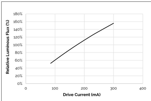
**Figure 4: V4B HD Typical Relative Luminous Flux vs. Drive Current ( $T_j = T_c = 25^\circ\text{C}$ )<sup>1</sup>**
