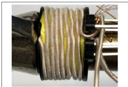
Figure 17 Secondary part of the primary winding
