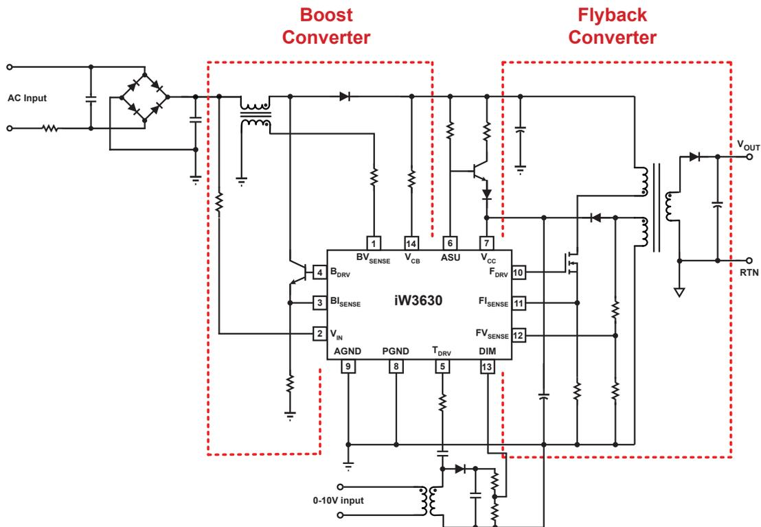
Figure 3.2 : iW3630 0-10V Dimming Simplified Schematic
