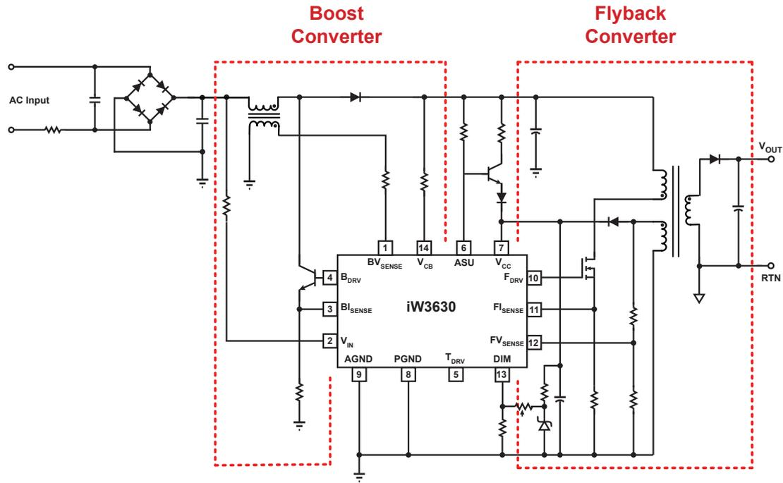
Figure 3.1 : iW3630 Analog Dimming Simplified Schematic
