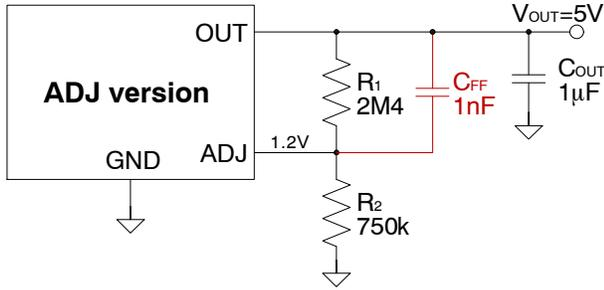
Figure 56. ADJ Output Voltage Schematic –  $C_{FF}$  Capacitor
