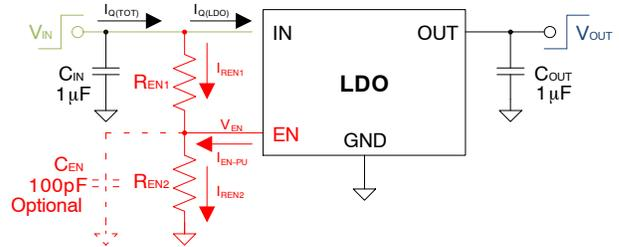
**Figure 74. Circuit – IN Voltage UVLO by EN Pin**
