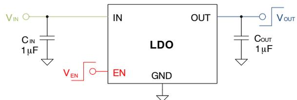
Figure 66. Circuit – LDO Controlled by  $V_{EN}$
