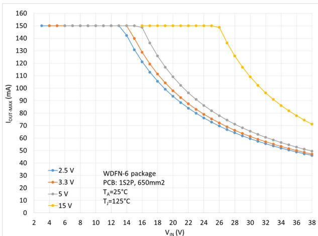
Figure 86. Maximum Output Current vs. Input Voltage
