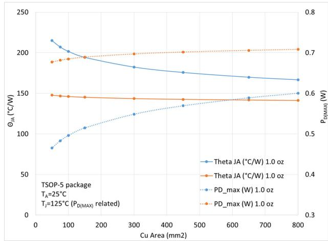
Figure 85.  $\theta_{JA}$  and  $P_{D(MAX)}$  vs. Copper Area
