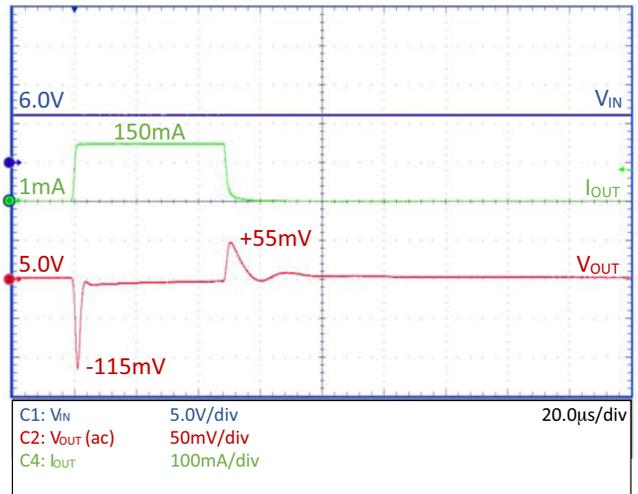
Figure 23. Load Transient – NCV8730–5.0 V,
