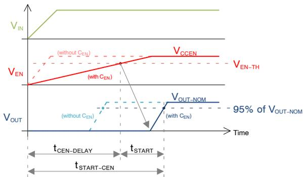
**Figure 69. Timing –  $C_{EN}$ -Delayed  $V_{IN}$ -Startup**
