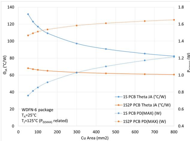
Figure 84.  $\theta_{JA}$  and  $P_{D(MAX)}$  vs. Copper Area
