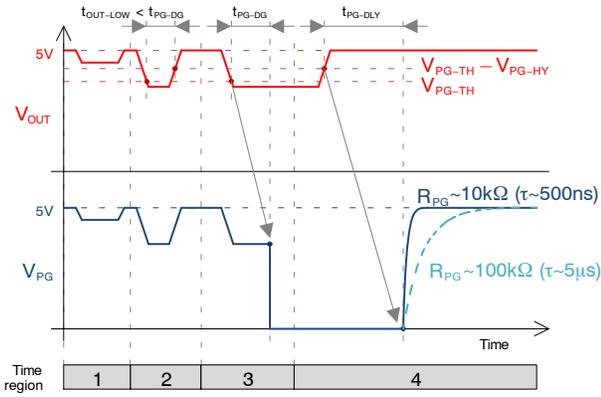
Figure 80. Timing – PG Connected to LDO’s Output
