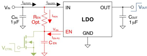
**Figure 72. Circuit – EN Pin with C<sub>EN</sub> Controlled by Transistor**
