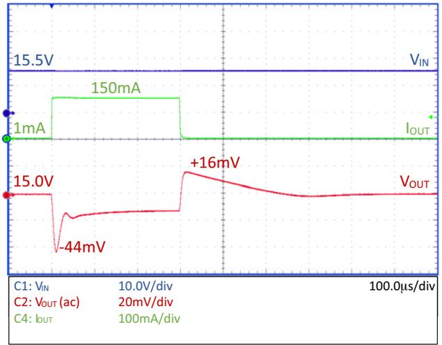
**Figure 31. Load Transient – NCV8730–15.0 V,
