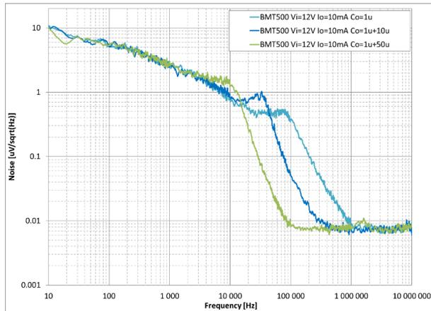
Figure 50. Noise – FIX – 5.0 V,  $I_{OUT} = 10\text{ mA}$ , Different  $C_{OUT}$
