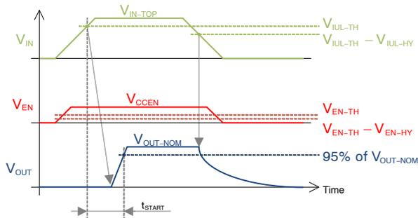
Figure 63. Startup Timing – Floating EN Pin
