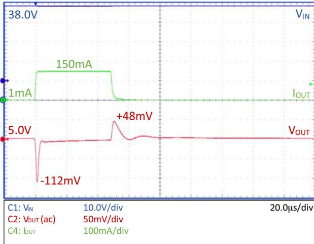
Figure 24. Load Transient – NCV8730–5.0 V,
