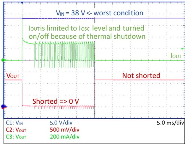
Figure 41. Output Short (20 ms) – NCP730–ADJ–1.2 V
