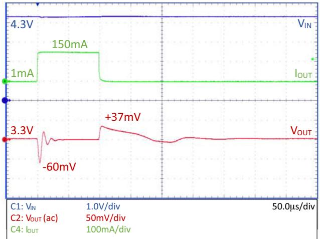
Figure 21. Load Transient – NCV8730–3.3 V,
