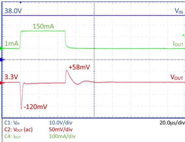
Figure 20. Load Transient – NCV8730–3.3 V,
