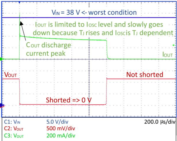
Figure 40. Output Short (1 ms) – NCP730–ADJ–1.2 V
