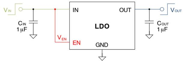
Figure 64. Circuit – EN Pin Connected to IN Pin
