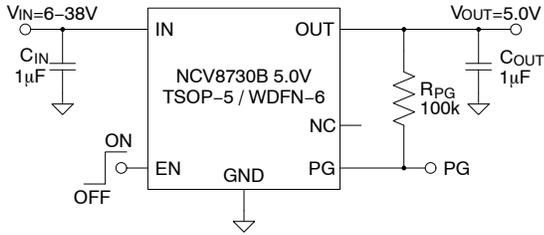
Figure 3. Fixed Output Voltage Application with PG
