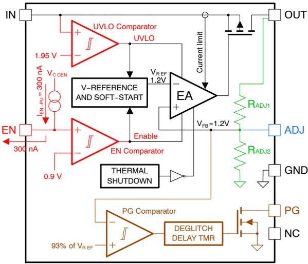
Figure 61. Internal Block Diagram – EN Pin
