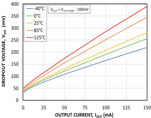
Figure 16. NCV8730BMT500 - Dropout Voltage
