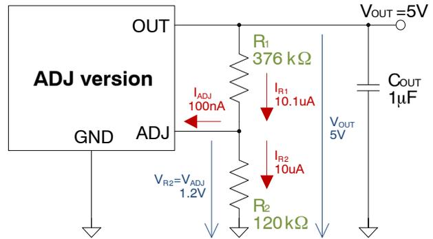
Figure 55. ADJ Output Voltage Schematic – Example 2
