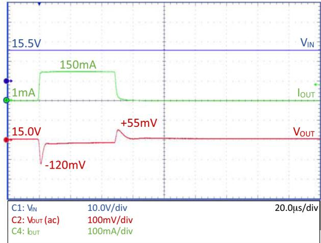
Figure 27. Load Transient – NCV8730–15.0 V,
