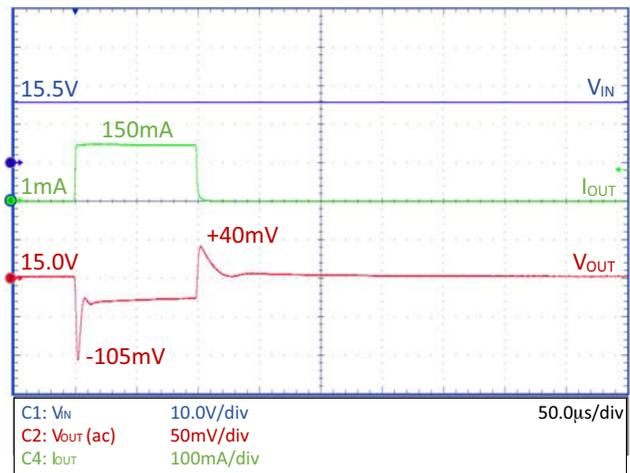
Figure 29. Load Transient – NCV8730–15.0 V,
