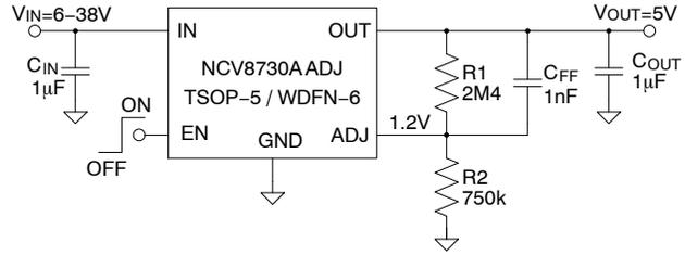
Figure 2. Adjustable Output Voltage Application (No PG)
