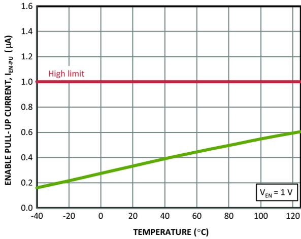
Figure 12. Enable Internal Pull-Up Current vs. Temperature
