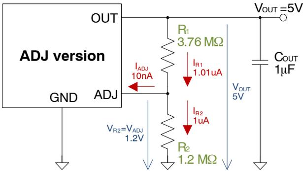
Figure 54. ADJ Output Voltage Schematic – Example 1
