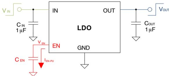
**Figure 68. Circuit –  $C_{EN}$ -Delayed  $V_{IN}$ -Startup**
