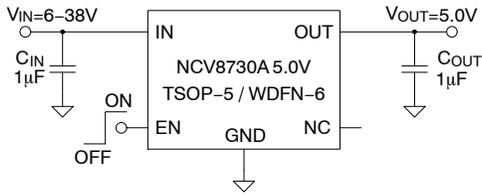
Figure 1. Fixed Output Voltage Application (No PG)
