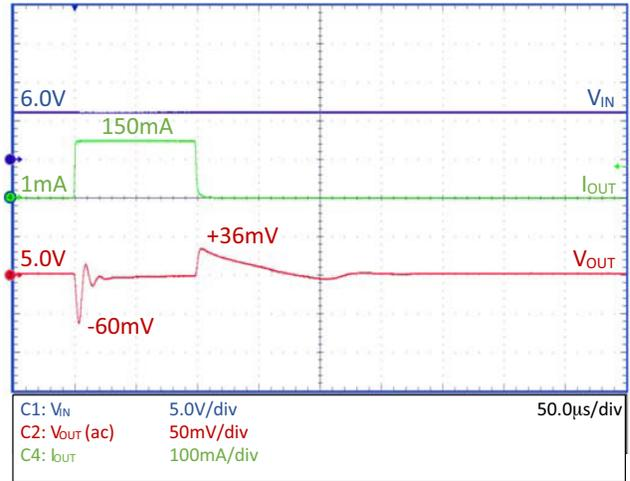
Figure 25. Load Transient – NCV8730–5.0 V,
