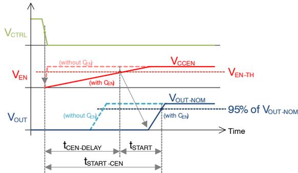
**Figure 73. Startup Timing – EN Pin with C<sub>EN</sub> Controlled by Transistor**
