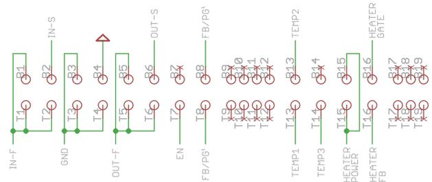
**Figure 88. Edge Connector Pinout (All Demo Boards)**
