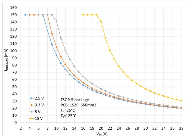
Figure 87. Maximum Output Current vs. Input Voltage
