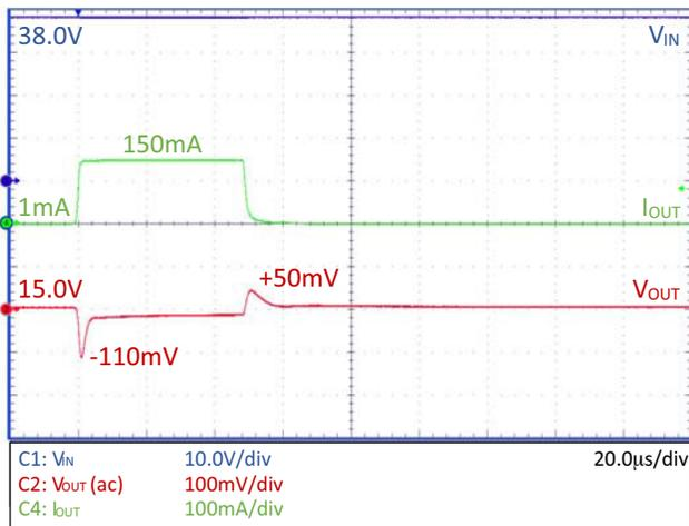
Figure 28. Load Transient – NCV8730–15.0 V,
