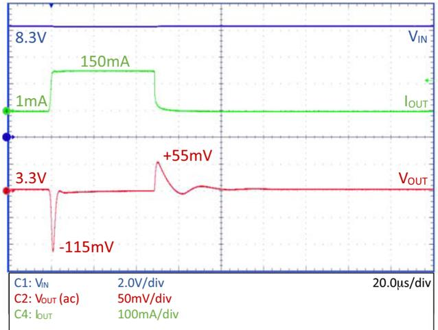
Figure 19. Load Transient – NCV8730–3.3 V,
