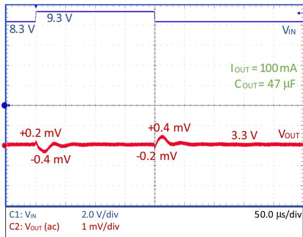
Figure 39. Line Transient – NCP730–3.3 V
