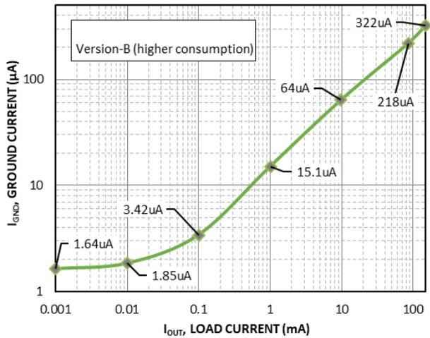
Figure 7. Ground Current vs. Load (NCP730-5.0V, Version-B)
