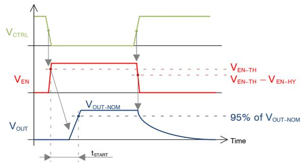
**Figure 71. Startup Timing – EN Pin Controlled by Transistor**
