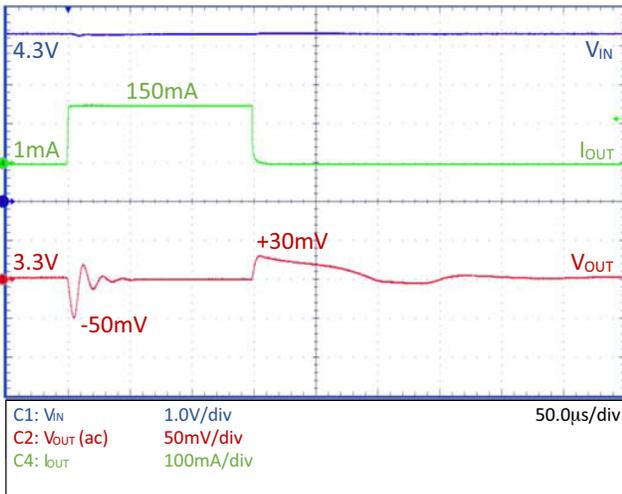
Figure 22. Load Transient – NCV8730–3.3 V,
