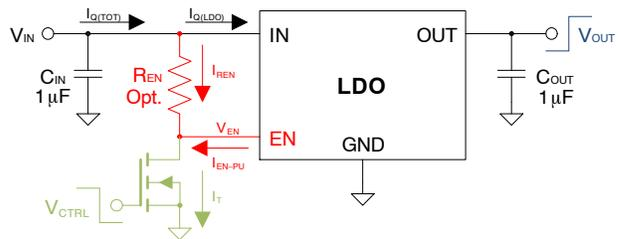
**Figure 70. Circuit – EN Pin Controlled by Transistor**
