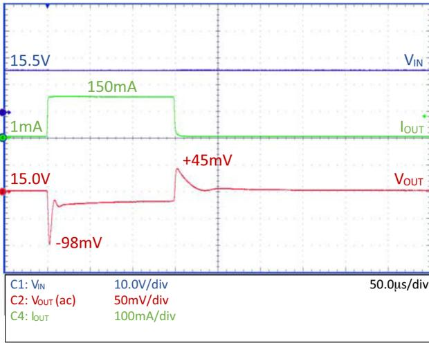
**Figure 30. Load Transient – NCV8730–15.0 V,
