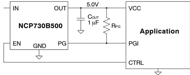
**Figure 78. Circuit Example – PG Connected to LDO's Output**
