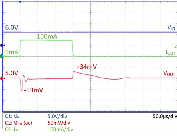
Figure 26. Load Transient – NCV8730–5.0 V,
