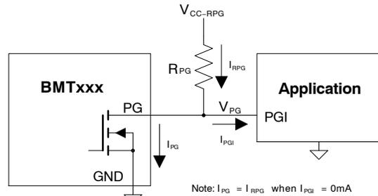
Figure 82. Circuit Example for  $R_{PG}$  Value Selection
