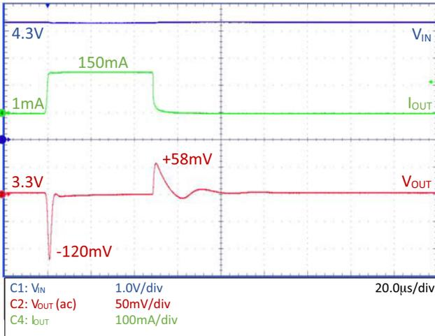
Figure 18. Load Transient – NCV8730–3.3 V,
