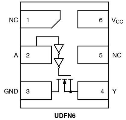
Figure 2. Pinout (Top View)
