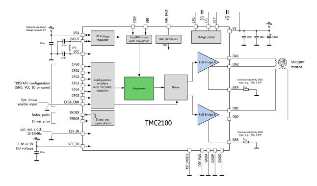
Figure 3.1 Standalone operation example circuit
