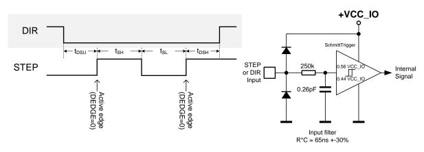
Figure 11.1 STEP and DIR timing, Input pin filter
