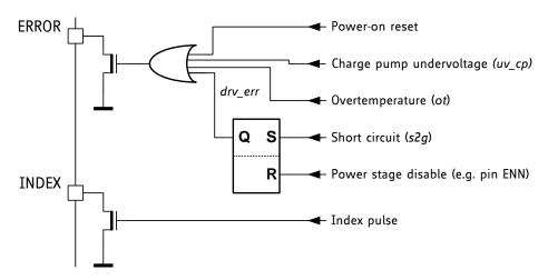
Figure 10.1 Error and Index output
