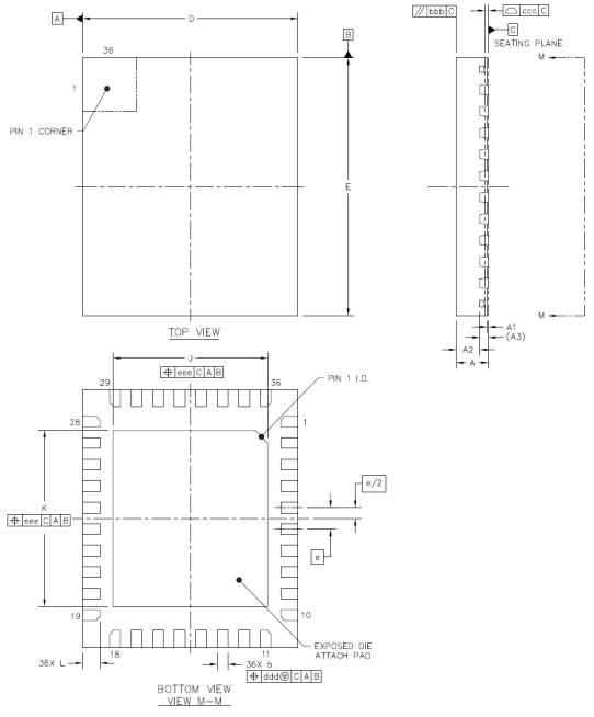
Figure 17.1 Dimensional drawings QFN 5x6
