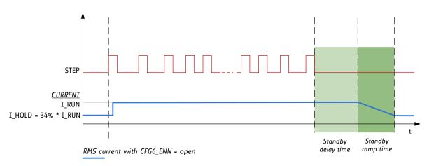
Figure 1.2 Standstill current reduction
