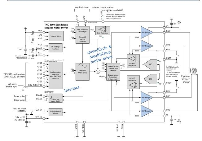
Figure 1.1 TMC2100 standalone driver application diagram
