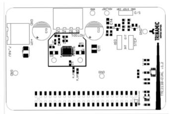
In this example, configuration is hard wired. The motor is driven via step and direction signals. Motion control tasks and interpreting ERROR and INDEX are software based.
