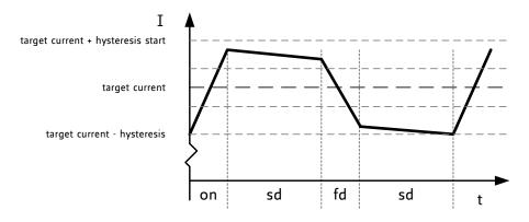
Figure 6.3 SpreadCycle chopper scheme showing coil current during a chopper cycle
