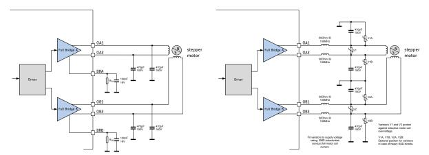
Figure 4.7 Simple ESD enhancement and more elaborate motor output protection
