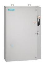
Non-reversing motor starter Size 1 Three phase full voltage Solid-state overload relay OLRelay amp range 5.5-22A 110VAC 50HZ / 120VAC 60HZ coil Combination type 30Amp non-fusible disconnect Encl NEMA type 4X 316 S-steel Water/dust tight non-corrosive Extra-wide enclosure
