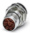
Device connector for rear wall, straight, shielded: yes, for standard and SPEEDCON interlock, M23, No. of pos.: 4+4+4+PE / 3+N+PE, type of contact: Socket, Crimp connection, Flat gasket, Central fastening M26 x 1, Panel thickness min.: 1.5 mm, Panel thickness max.: 5 mm
