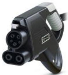
DC charging cable, DC charging cable with vehicle connector, open cable end, CCS type 1, Combined Charging System, SAE J1772, IEC 62196-3, 60 A / 600 V (DC), design line Standard, cable: 25 ft, black, straight, NOTE: Cable management may be required., mating face: black, handle area: gray
