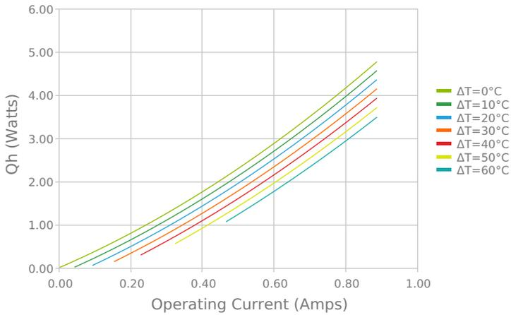
Total Heat Dissipated at Hot Side (Qh=Qc+Pin)
