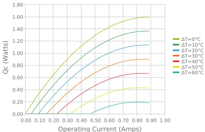
Heat Pumped at Cold Side
