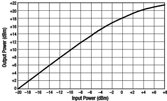
Figure 3. Output Power vs Input Power @ 2445 MHz
