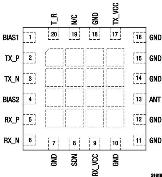
Figure 2. SKY65344-21 Pinout – 20-Pin MCM (Top View)
