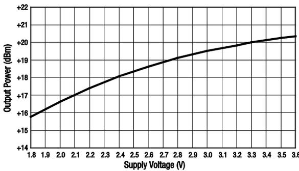
Figure 5. Output Power vs Supply Voltage @ 2445 MHz
