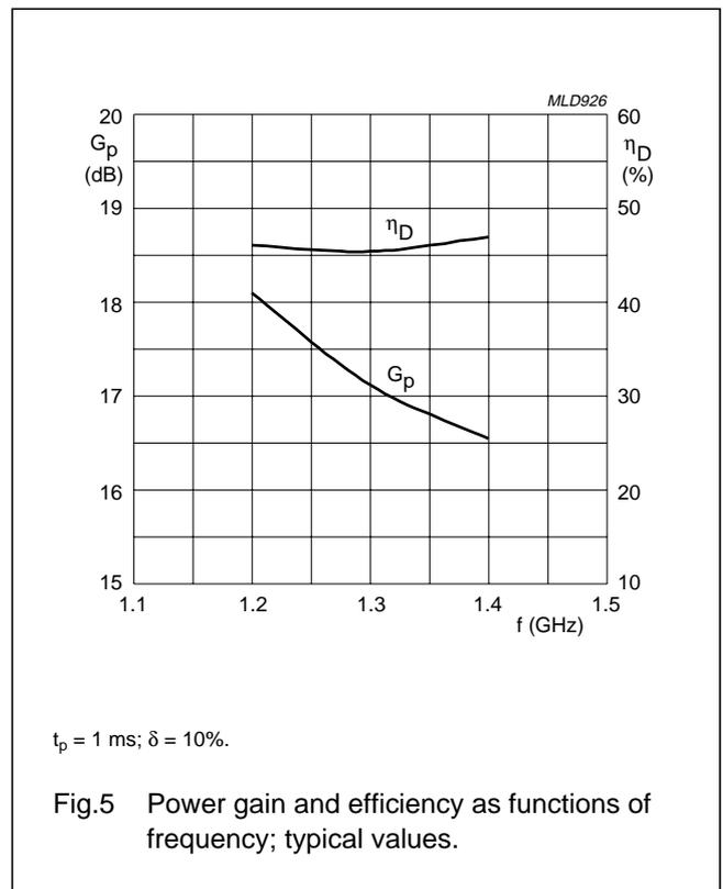
L-band radar LDMOS driver transistor
