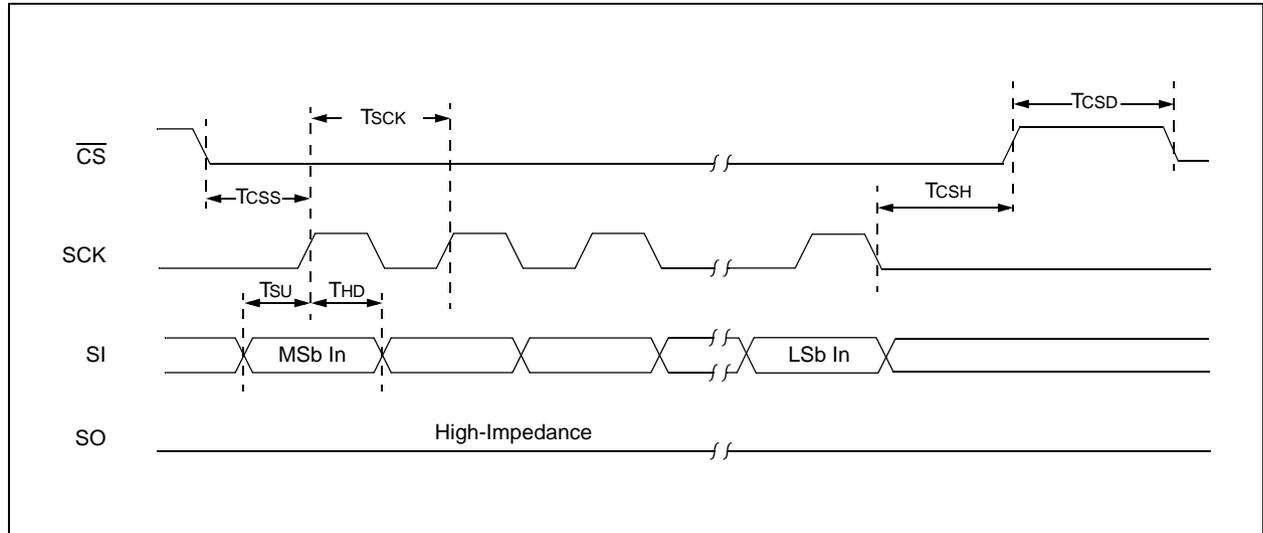
$\overline{\text{CS}}$  must be toggled for each SPI block transfer.
