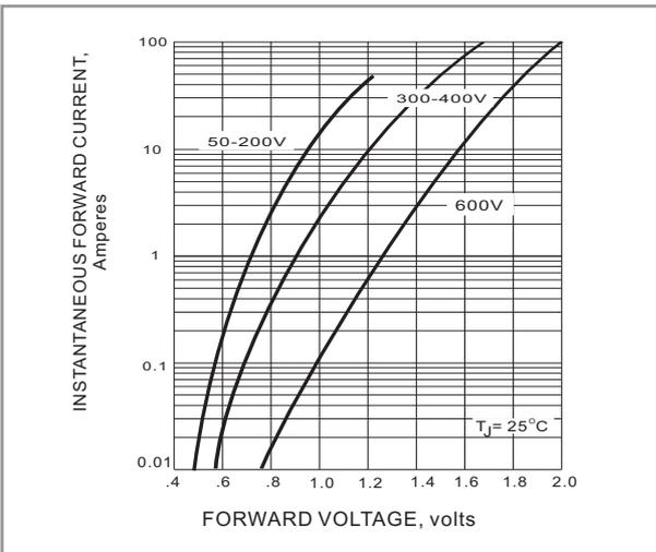
Fig.3 FORWARD CHARACTERISTICS
