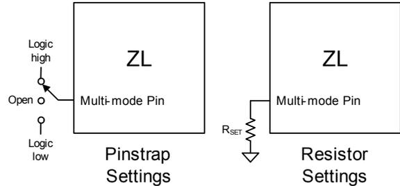
FIGURE 12. PIN-STRAP AND RESISTOR SETTING EXAMPLES
