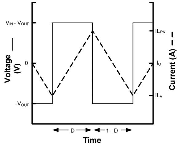
FIGURE 11. INDUCTOR WAVEFORM
