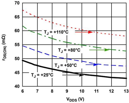
**FIGURE 7. LOW-SIDE  $r_{DS(ON)}$  vs  $V_{DD5}$  WITH  $T_J$**
