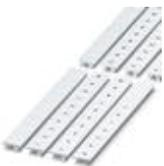
Marker for terminal blocks, Strip, white, labeled, can be labeled with: Plotter, Horizontal: L1, L2, L3, N, PE, L1, L2, L3, N, PE, Mounting type: Snap into tall marker groove, for terminal block width: 10.2 mm, Lettering field: 10.15 x 10.5 mm
