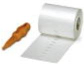
Marker for terminal blocks, Roll, white, unlabeled, can be labeled with: THERMOMARK ROLL, THERMOMARK ROLL X1, THERMOMARK X, THERMOMARK S1.1, Perforated, Mounting type: Snap into universal marker groove, Snap into flat marker groove, for terminal block width: 10.2 mm, Lettering field: 6.35 x 10.15 mm
