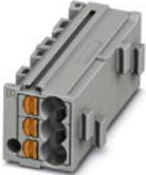
Marshalling patchboard, Nom. voltage: 500 V, Nominal current: 17.5 A, Cross section: 0.14 mm<sup>2</sup> - 2.5 mm<sup>2</sup>, AWG: 12 - 26, Connection type: Push-in connection, Number of positions: 1, Number of connections: 6, Width: 11 mm, Length: 12.2 mm, Color: gray, Color of connection elements: brown, Assembly: for snapping onto a DIN rail adapter, for snapping onto a cover flange
