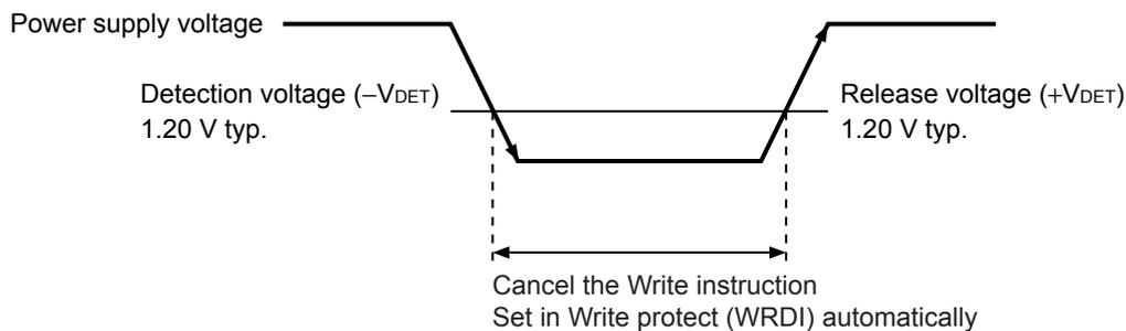
**Figure 21** Operation during Low Power Supply Voltage
