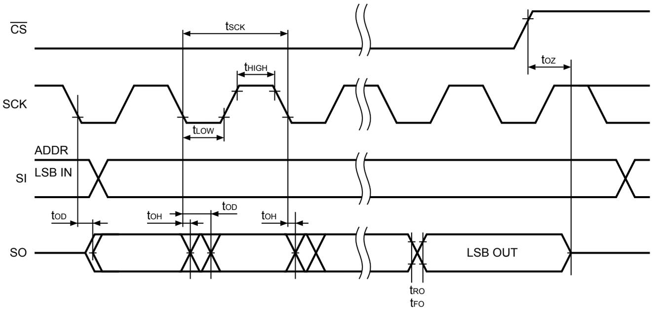
Figure 8 Serial Output Timing
