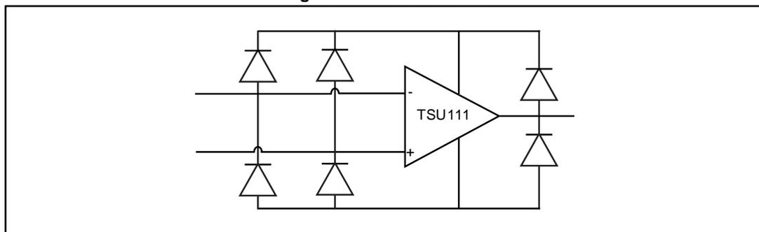
Current through the diodes must be limited to a maximum of 10 mA as stated in [Table 1: "Absolute maximum ratings \(AMR\)"](#). A serial resistor on the inputs can be used to limit this current.
