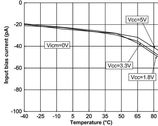
Figure 10: Input bias current vs. temperature at high VICM
