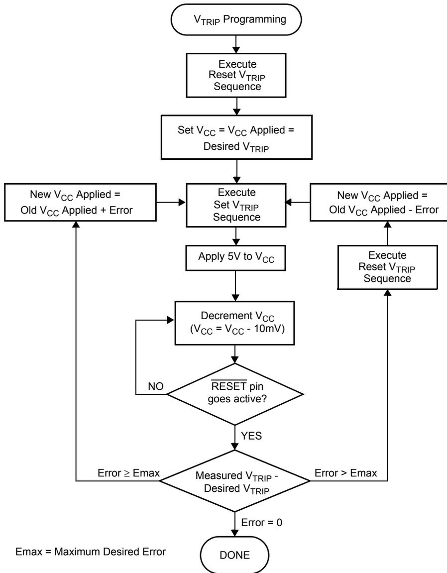
FIGURE 3. V<sub>TRIP</sub> PROGRAMMING SEQUENCE FLOW CHART
