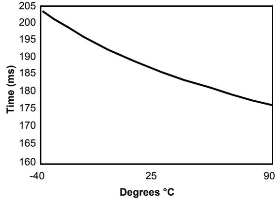
**V<sub>TRIP</sub> vs. Temperature (programmed at 25°C)**
