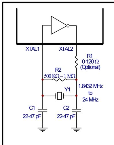
The on-chip oscillator is designed to use an industry standard microprocessor crystal (parallel resonant, fundamental frequency with 10-22 pF capacitance load, ESR of 20-120 ohms and 100 ppm frequency tolerance) connected externally between the XTAL1 and XTAL2 pins (see **Figure 4**). Alternatively, an external clock can be connected to the XTAL1 pin to clock the internal baud rate generator for standard or custom rates.
