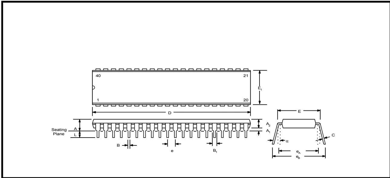
Note: The control dimension is the millimeter column
