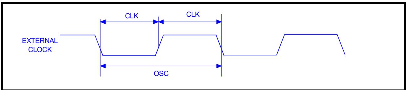
**FIGURE 17. MODEM INPUT/OUTPUT TIMING FOR CHANNELS A & B**
