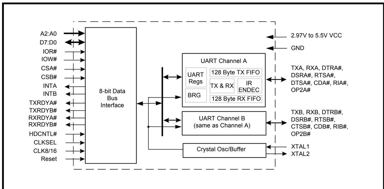
**FIGURE 2. PIN OUT ASSIGNMENT**
