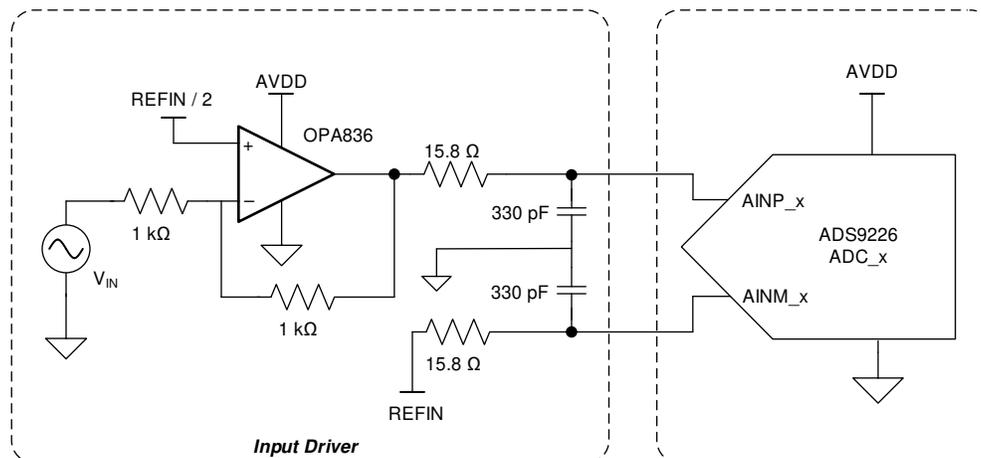
**Figure 8-2. Typical Connection Diagram of the ADS9226 Application Circuit**
