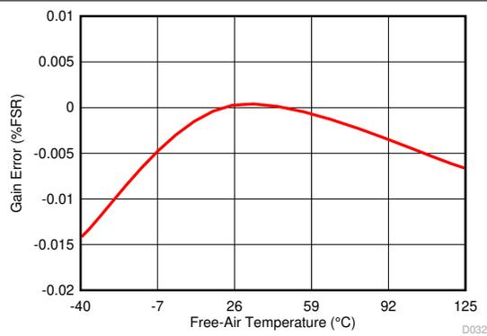
**Figure 6-14. Gain Error vs Free-Air Temperature**
