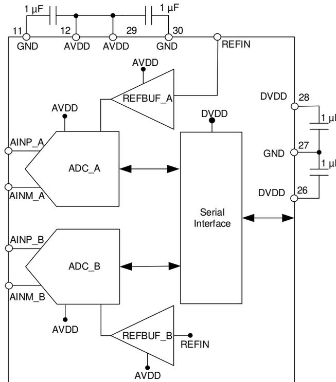
**Figure 9-1. Power-Supply Decoupling**
