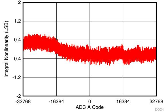
**Figure 6-17. Typical INL ADC A**
