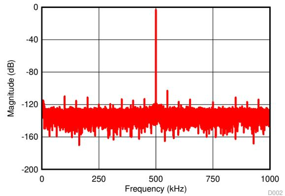
$f_{\text{IN}} = 500\text{ kHz}$ , SNR = 90 dB, THD = -90.9 dB
