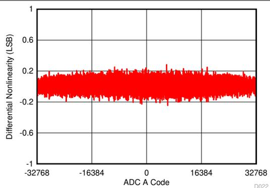
**Figure 6-15. Typical DNL ADC A**
