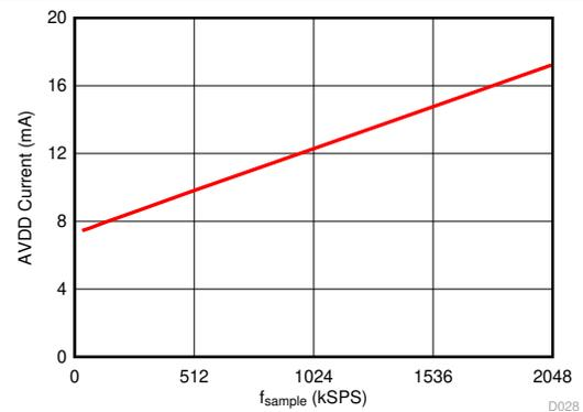
**Figure 6-21. Dynamic AVDD Current vs Sampling Rate**
