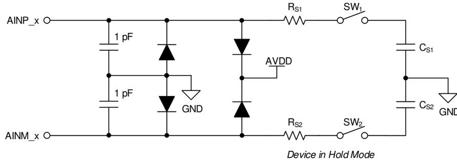
**Figure 7-2. Analog Input Structure for Converter Module**
