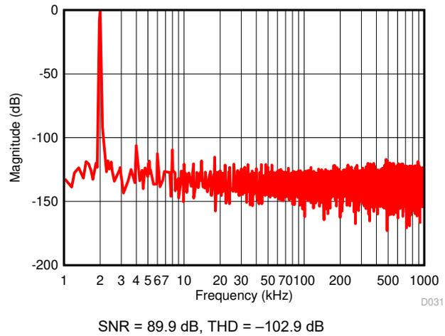
**Figure 8-3. Typical FFT With a 2-kHz Signal**
