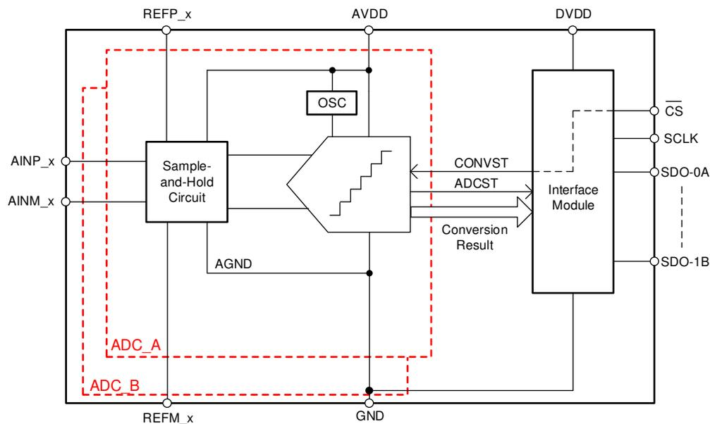
**Figure 7-1. Converter Modules**
