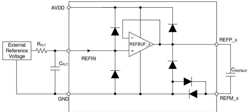
**Figure 7-4. Connection Diagram for Reference and Reference Buffers**
