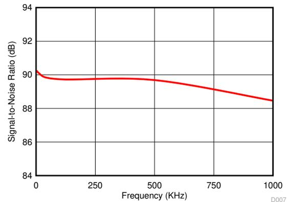
**Figure 6-9. SNR vs Input Frequency**
