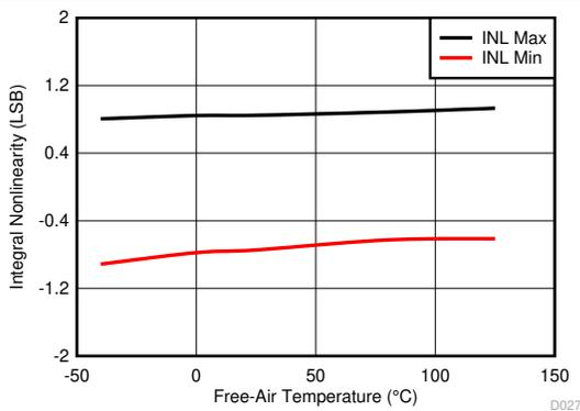
**Figure 6-20. INL vs Free-Air Temperature**
