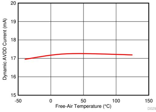
**Figure 6-22. Dynamic AVDD Current vs Free-Air Temperature**
