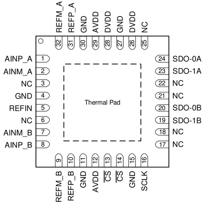
**Figure 5-1. RHB Package, 5-mm × 5-mm, 32-Pin VQFN, Top View**
