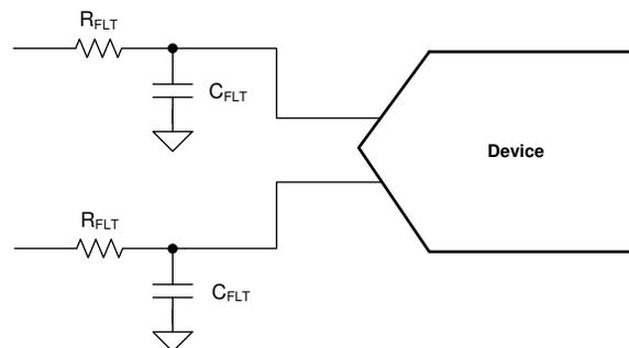
**Figure 8-1. Charge-Kickback Filter**
