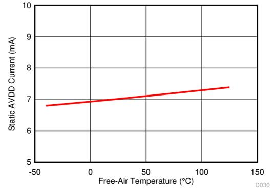
**Figure 6-23. Static AVDD Current vs Free-Air Temperature**
