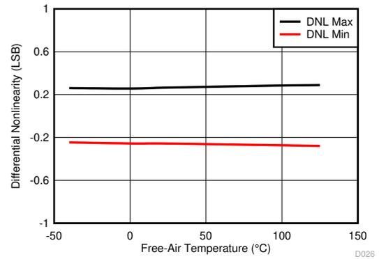
**Figure 6-19. DNL vs Free-Air Temperature**
