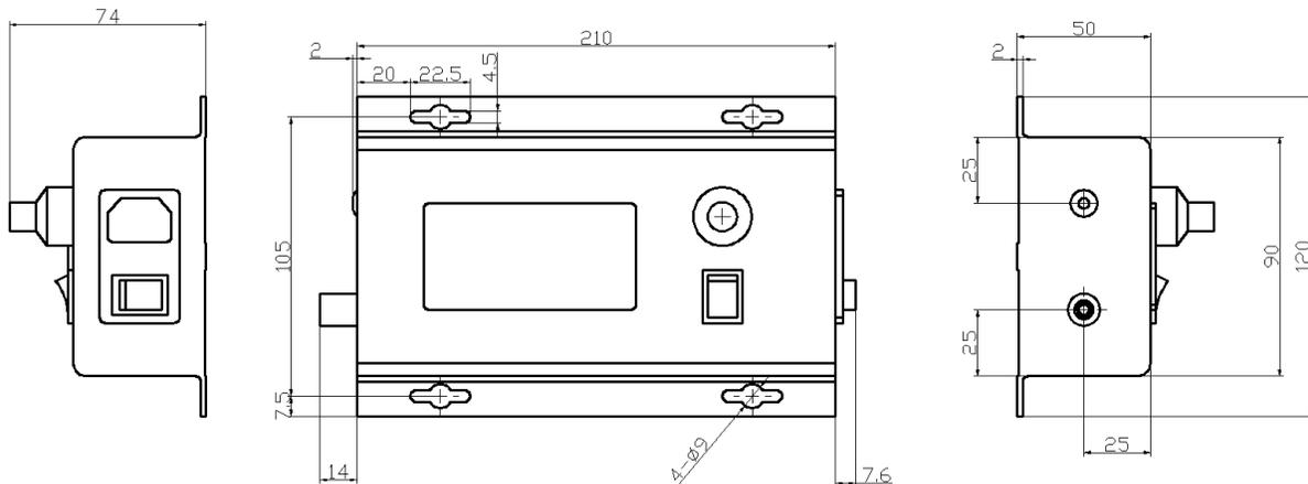
Figure 9. Dimensions for AHVACN5KV5MABT
