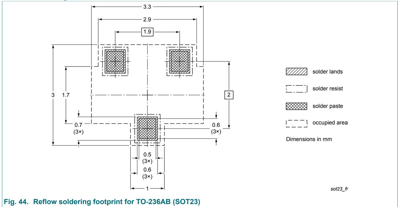
Fig. 44. Reflow soldering footprint for TO-236AB (SOT23)
