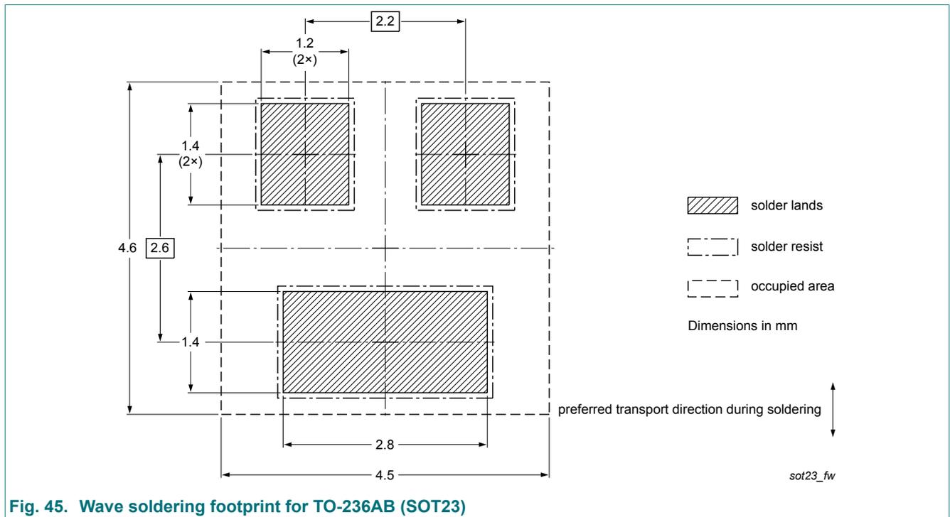
Fig. 45. Wave soldering footprint for TO-236AB (SOT23)
