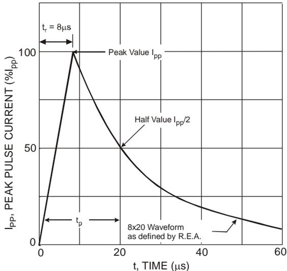
Figure 3 Pulse Waveform
