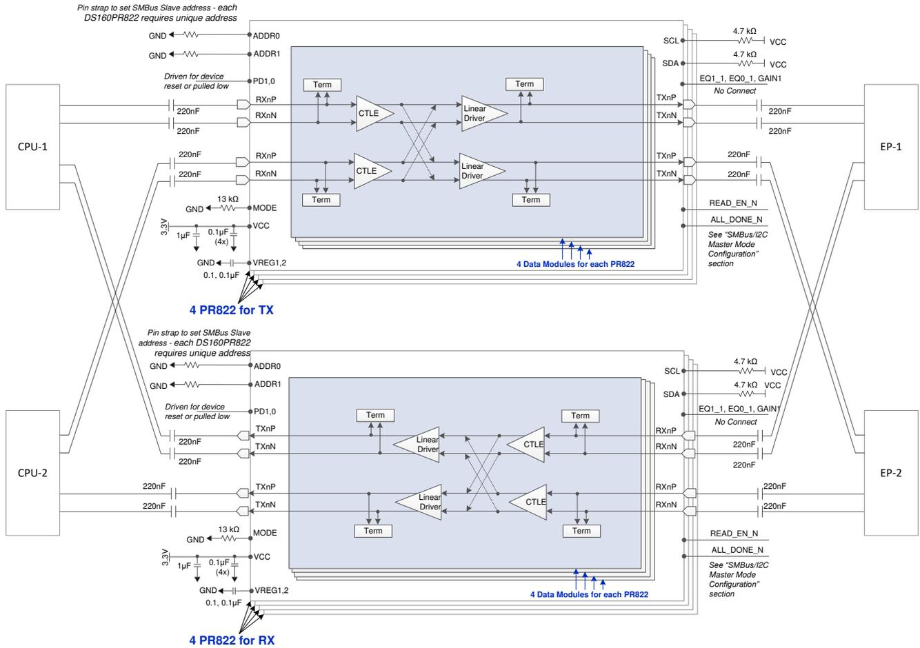
**Figure 8-3. Simplified Schematic for Lane Configuration in SMBus/I<sup>2</sup>C Master Mode**
