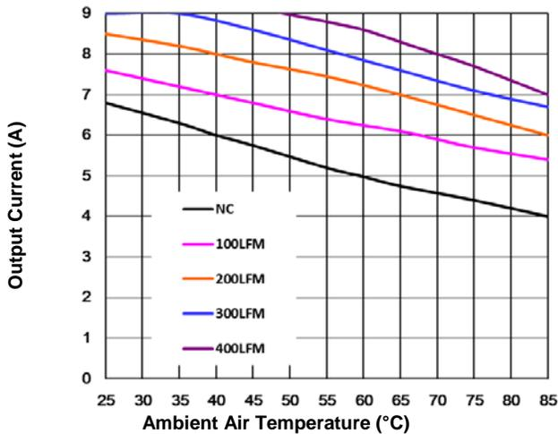
**Figure 9. Current Derating Curve for Airflow Direction 3**
