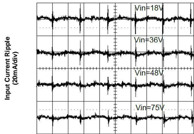
Figure 6. Input Reflected Ripple Current at Full Load
