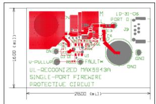
Figure 4. Single-port PCB top copper.
