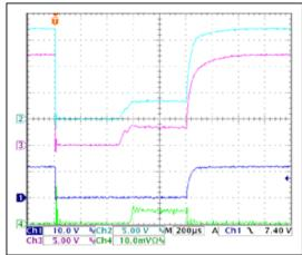
Figure 9A. Reference waveform showing the effects of an applied output short circuit with no simulated shorts applied to N2A, N2B, Q1A, or Q1B. CH1 =  $V_{OUT}$ , CH2 =  $N2B_{GATE}$ , CH3 =  $N2A_{GATE}$ , and CH4 =  $I_{OUT}$  (5A/div).
