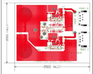
Figure 7. Dual-port PCB top copper.
