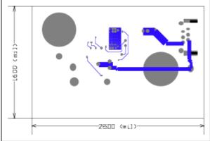
Figure 5. Single-port PCB bottom copper.
