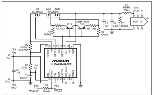
Figure 1. The connections required for Maxim's UL Recognized single-port FireWire protective circuit.
