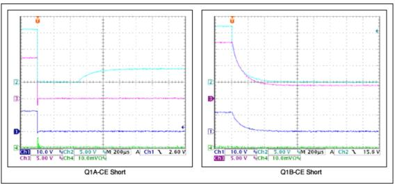
Figure 9C. Waveforms showing the effects of a Q1A or Q1B collector-emitter short. Predicted operation is verified.
