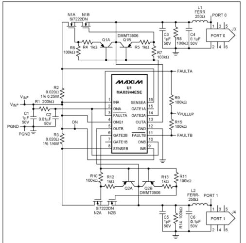
Figure 2. The connections required for Maxim's UL Recognized dual-port FireWire protective circuit.
