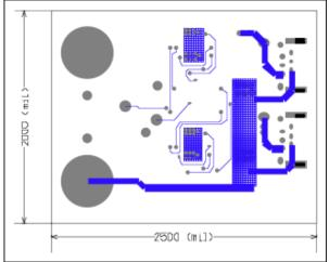
Figure 8. Dual-port PCB bottom copper.
