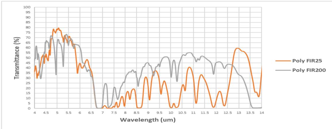
(Graph3 – Transmittance of PIR, FIR(Far infrared) material)
