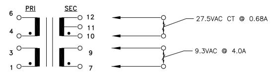
Required Secondary Fusing. Winding (7-9): T4.00A Winding (10-12): T0.80A
