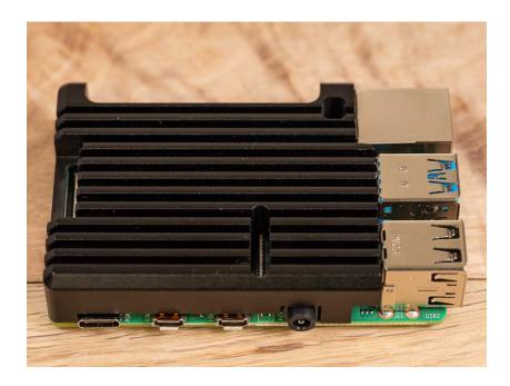
Flip the whole thing over, position the bottom case (make sure the mounting holes are the right way round), and then screw in the four hex bolts using the little allen key that's included.
