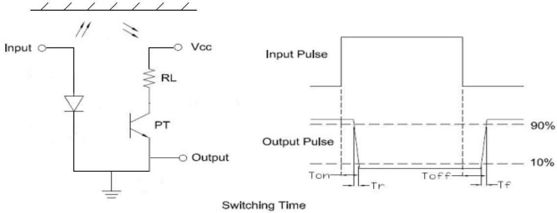
■ **Light Current Measurement Setup Diagram**
