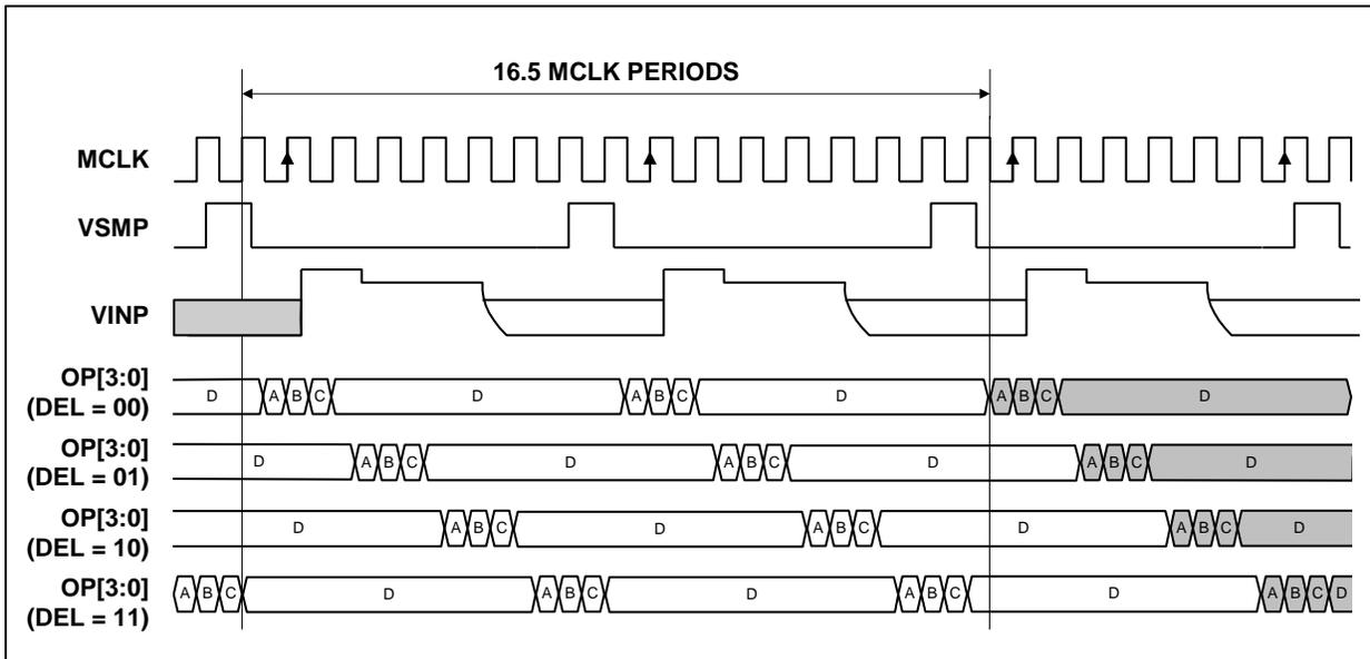
Figure 21 Mode 4 Operation (MCLK:VSMP Ratio = 8:1)
