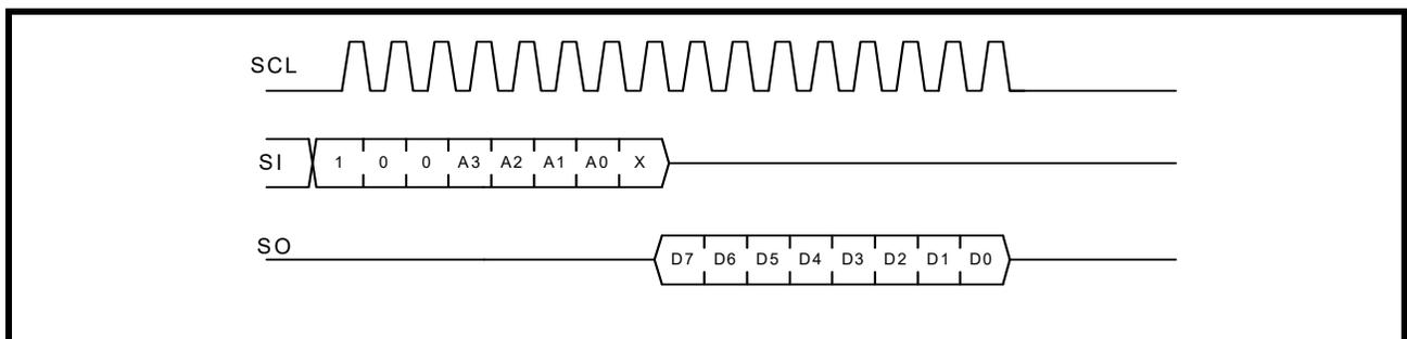
After the last read or write transaction, the SPI master will set the SCL signal back to its idle state (LOW).
