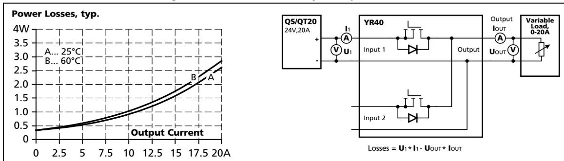
**Note:** As soon as voltage is applied on input 2, an additional 0.35W will be consumed. It is not relevant, whether this channel contributes to the output current or not.
