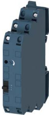
Signal converter with Manual-Auto switch 24-240 V AC/DC, 3-way separation input: 0-10 V, 0/4-20 mA output: 0-10 V, 0/4-20 mA screw terminal
