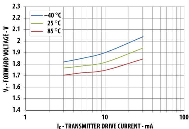
Figure 2. Typical forward voltage vs. drive current
