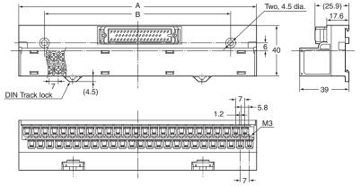
Note: There is only one DIN Track lock located in the center of the terminal block for a 20-pole Unit.
