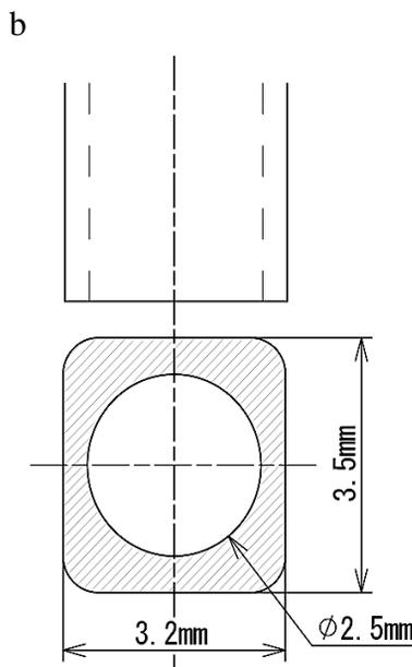
※Nozzle with chamfering is recommended
