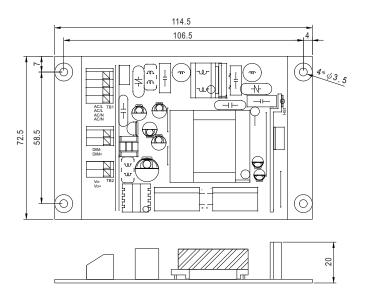
NOTE: Please use wires with a cross section of 0.75~1.5mm $^2$  for TB1 and wires with a cross section of 0.5~1.5mm $^2$  for TB2.
