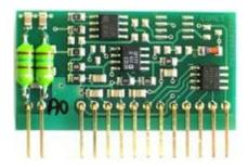
Accuracy -140 to+100°C  $\pm 0.2$ °C 100 to 600°C  $\pm 0.2$ % from reading. Galvanically unisolated. Two-wire connection.
