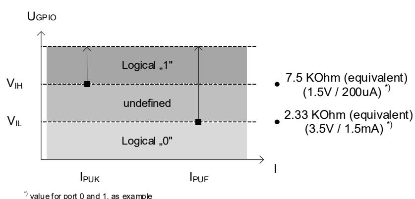
**Figure 46** Pull-Up Keep and Forced Current
