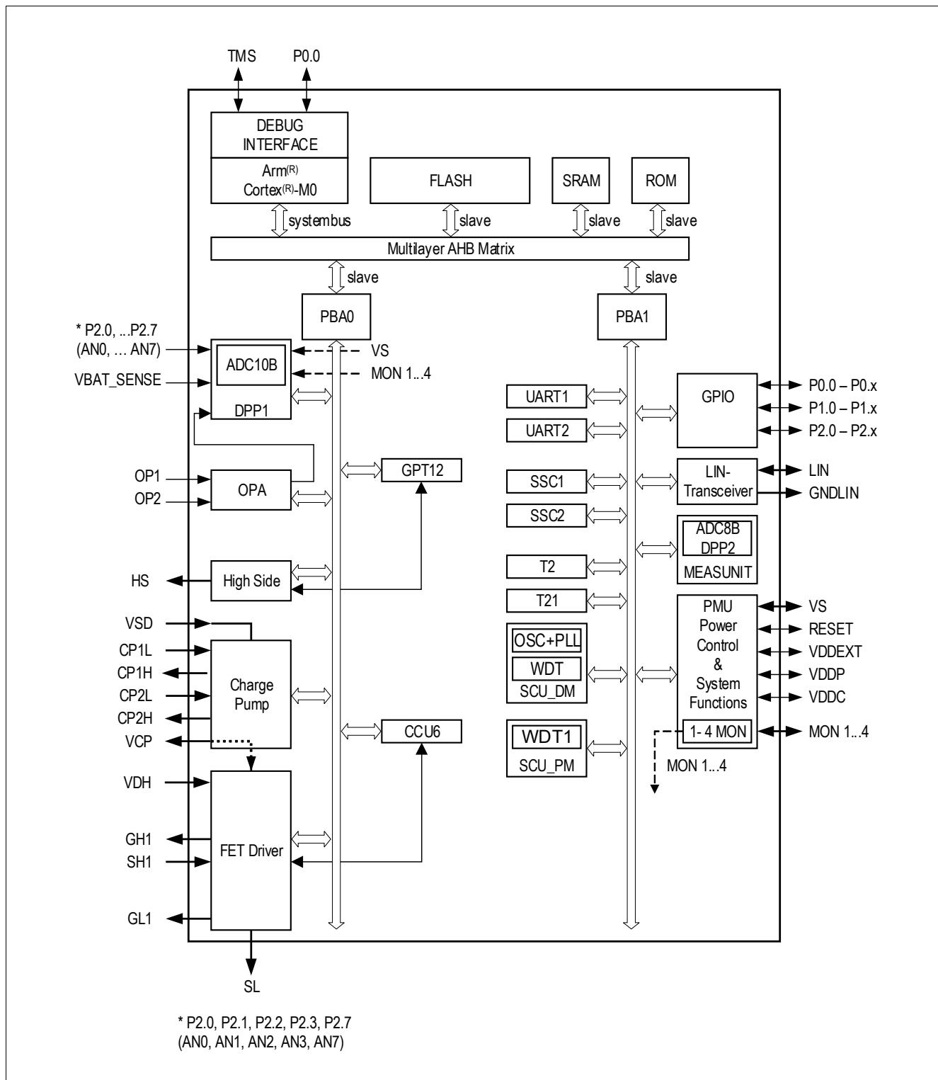
**Figure 1 Block Diagram TLE9851QXW**
