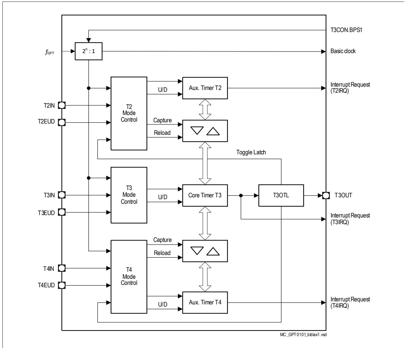
Figure 22 GPT1 Block Diagram ( $n = 2 \dots 5$ )
