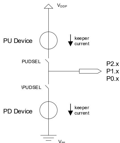
**Figure 45** Pull-Up/Down Device
