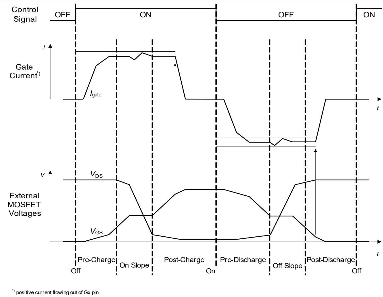
**Figure 34** Switching cycle
