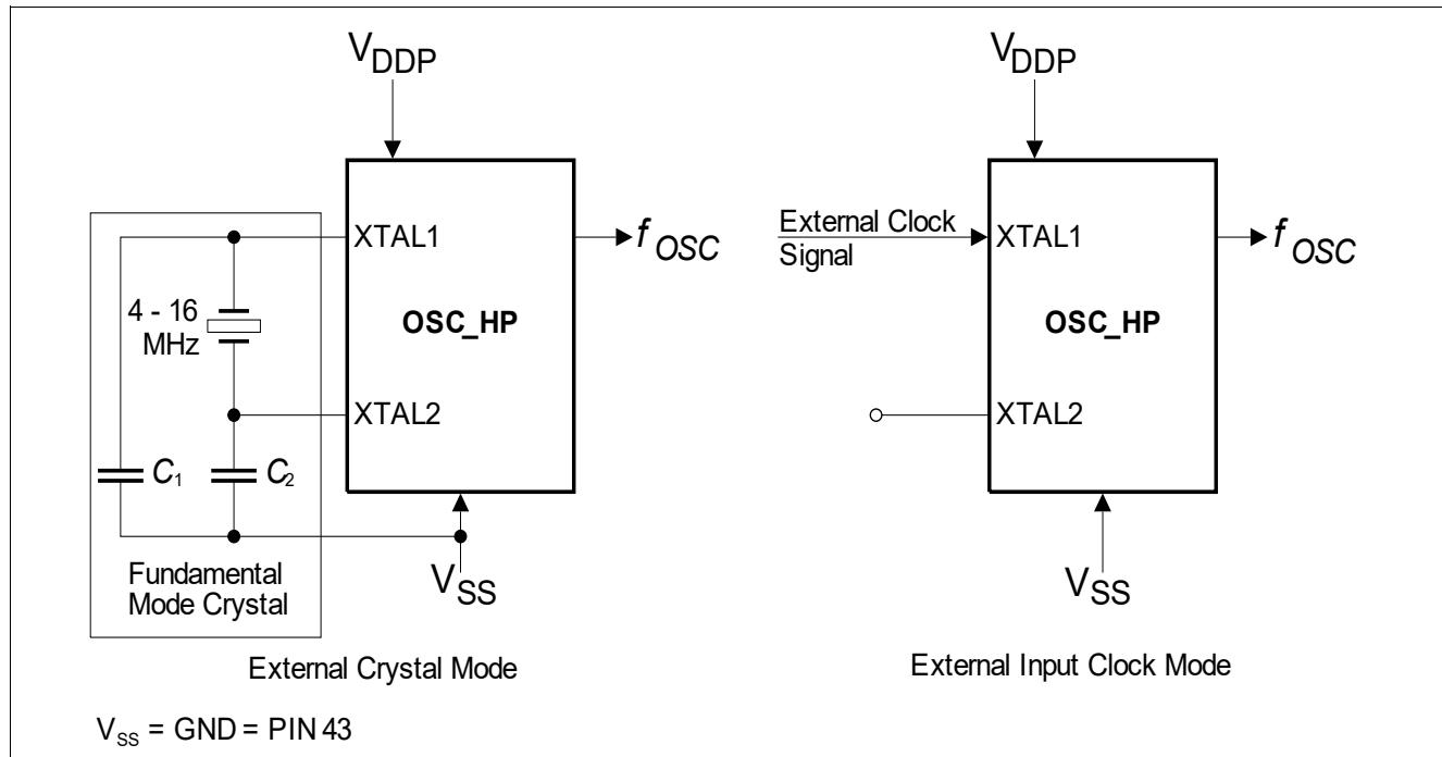
**Figure 11 TLE9851QXW External Circuitry for the OSC\_HP**
