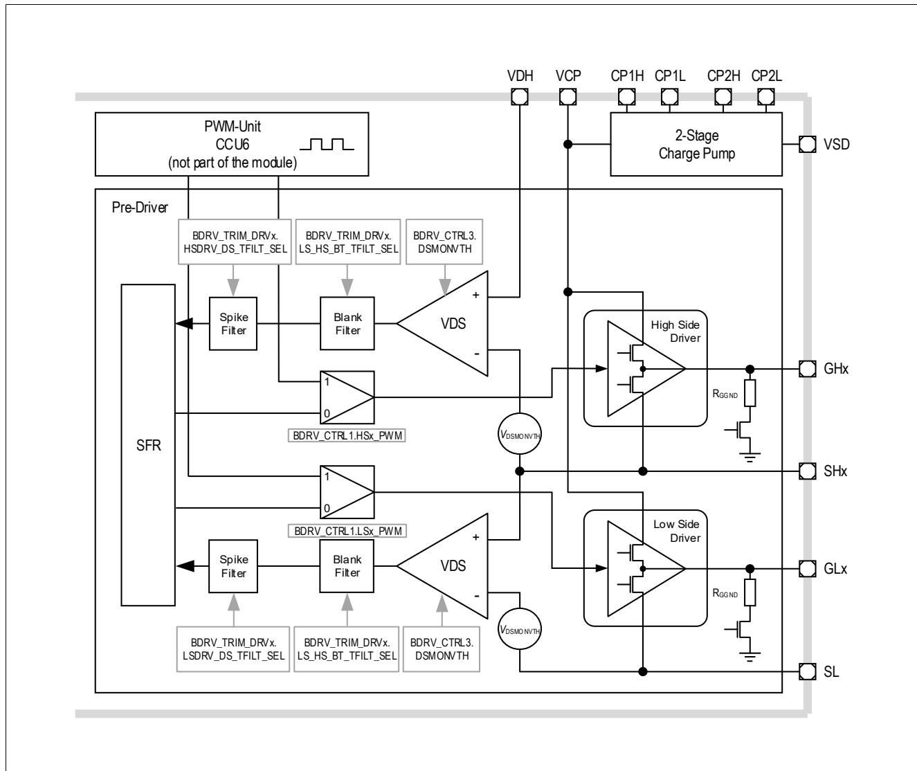
Figure 33 Driver Module Block Diagram (incl. System Connections)
