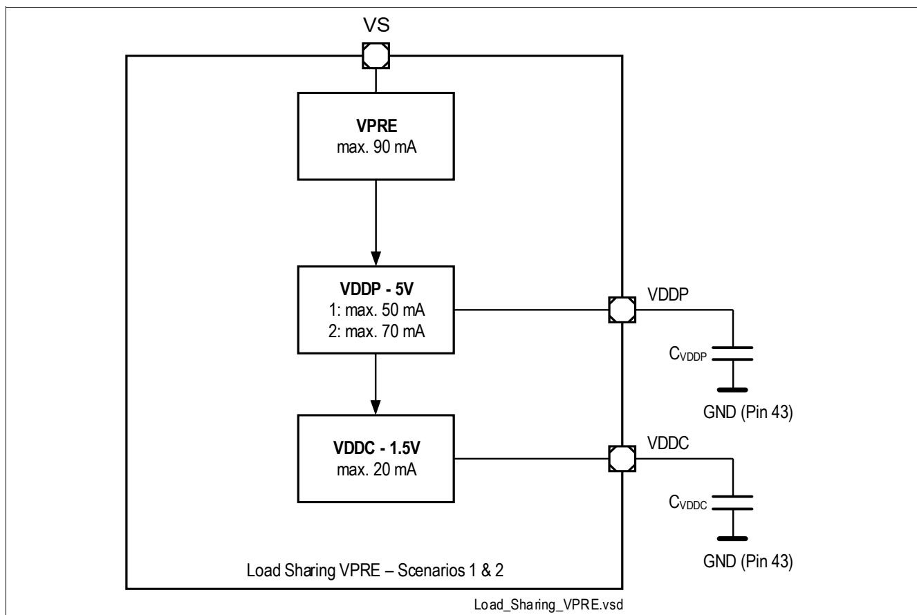
**Figure 44 Load Sharing Scenario of VPREG and VDDP Regulator**
