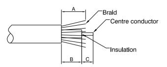
2) Tin the centre conductor. Slide the clamp nut, washer and grommet over the cable. Place the taper clamp over the braid and push back against the cable jacket. Pull the braid back over the taper clamp and trim level with the rear as shown.
