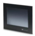
Touch panel with 38.1 cm/15" TFT-Display (Analog resistive (polyester)), 1024 x 768 Pixel (XGA), 256 colors, Xscale® PXA320, 806 MHz, 2x USB host 1.1, 1x CompactFlash®, 1 x Ethernet (10/100 Mbps), RJ45, Windows CE 6.0 and User software: Visu+ / AX OPC Server. (Bus system: without)
