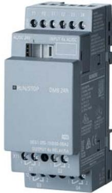
LOGO! DM8 24R expansion module, PS/I/O: 24V/24V/relay, 2 MW 4 DI/4 DO, AC/DC/NPN input for LOGO! 8
