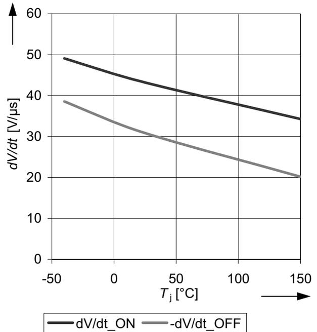
**Figure 30** Typical slew rate for turn ON  $(dV/dt)_{ON}$  and turn OFF  $-(dV/dt)_{OFF}$  as a function of the junction temperature  $T_j$
