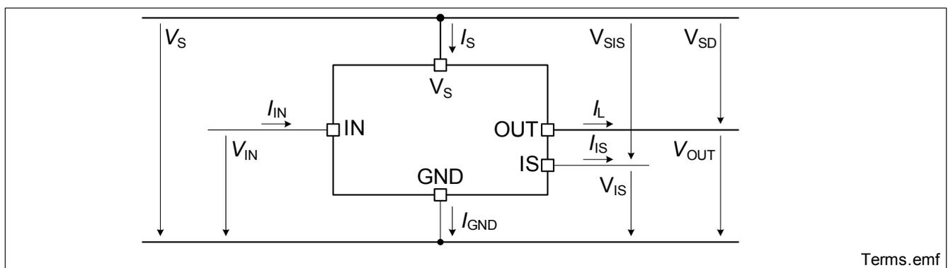
Figure 3 Definition of currents and voltages
