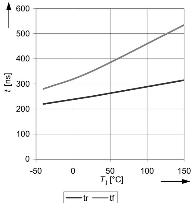
**Figure 32** Typical turn ON rise time  $t_r$  and and turn OFF fall time  $t_f$  as a function of the junction temperature  $T_j$
