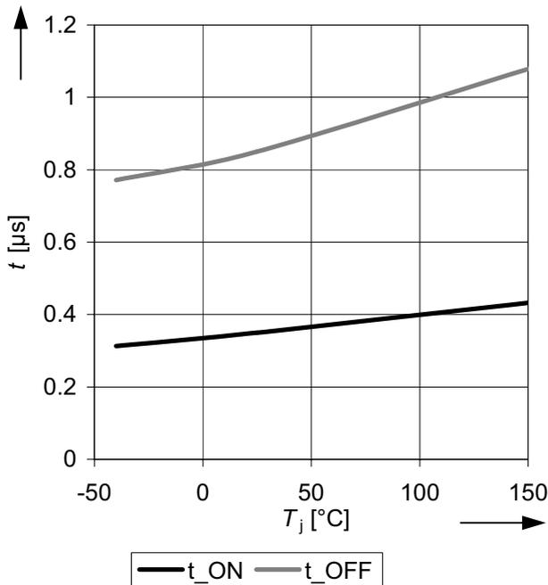
**Figure 31** Typical turn ON time  $t_{ON}$  and and turn OFF time  $t_{OFF}$  as a function of the junction temperature  $T_j$
