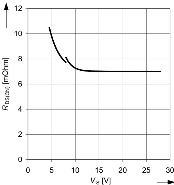
**Figure 27** Typical ON state resistance  $R_{DS(ON)}$  as a function of the supply voltage  $V_S$
