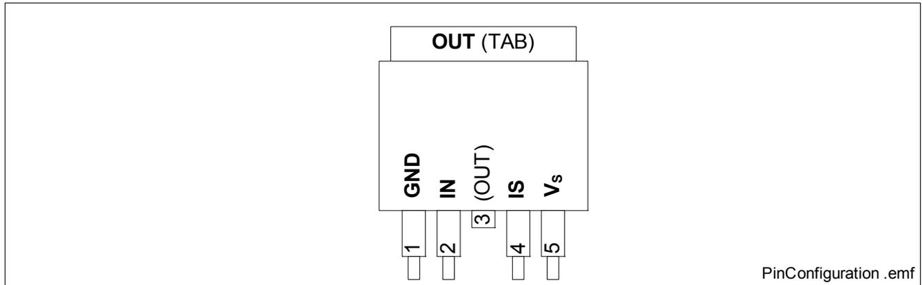
Figure 2 Pin Configuration
