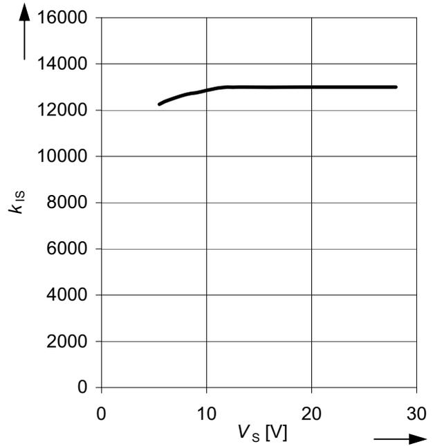
**Figure 39** Typical sense current slope  $k_{IS}$  as a function of the supply voltage  $V_S$
