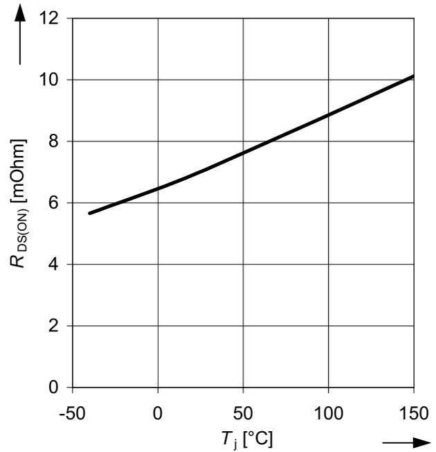
**Figure 26** Typical ON state resistance  $R_{DS(ON)}$  as a function of the junction temperature  $T_j$
