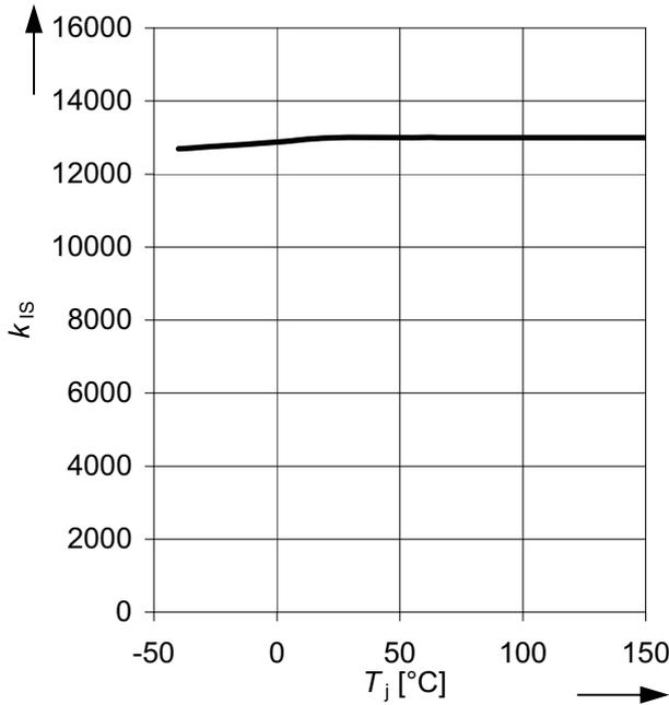
**Figure 38** Typical sense current slope  $k_{IS}$  as a function of the junction temperature  $T_j$
