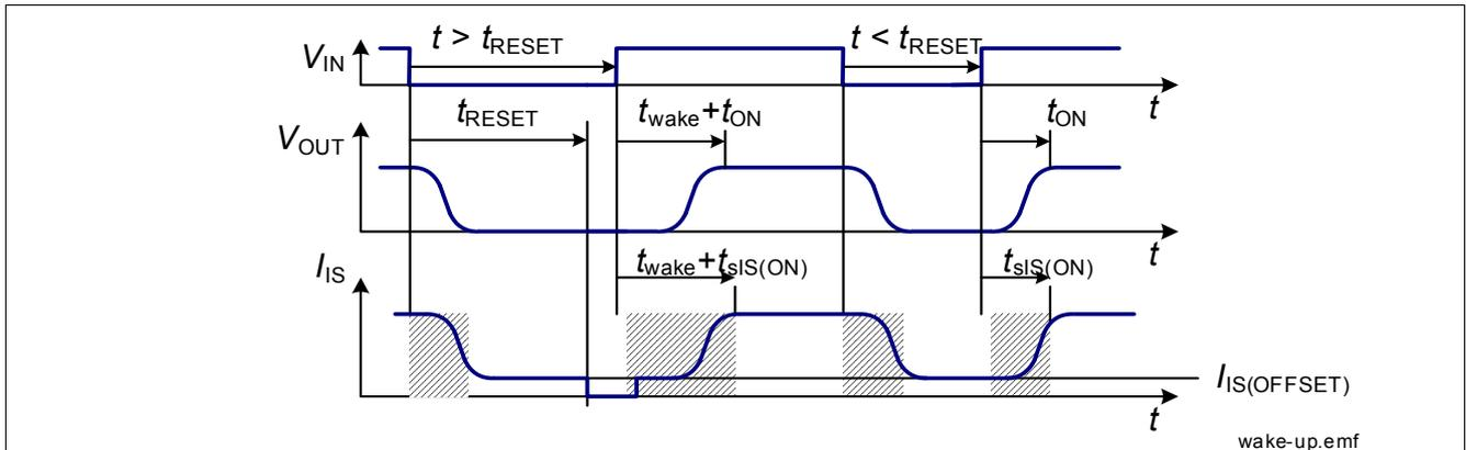
Figure 11 Wake up timing
