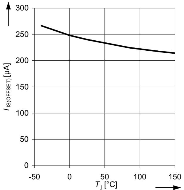
**Figure 41** Typical sense current offset  $I_{IS(OFFSET)}$  as a function of the junction temperature  $T_j$
