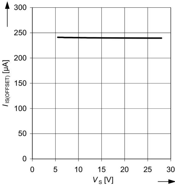
**Figure 42** Typical sense current offset  $I_{IS(OFFSET)}$  as a function of the supply voltage  $V_S$
