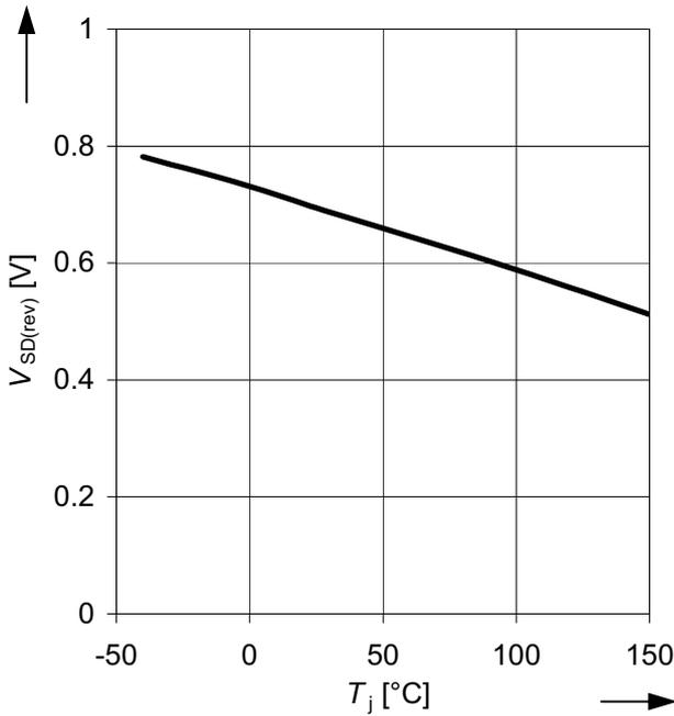
**Figure 29** Typical body diode forward voltage drop  $-V_{SD(rev)}$  as a function of the junction temperature  $T_j$
