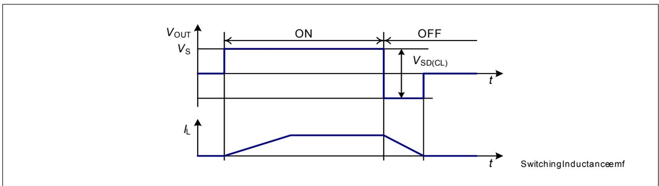
Figure 12 Switching an inductance
