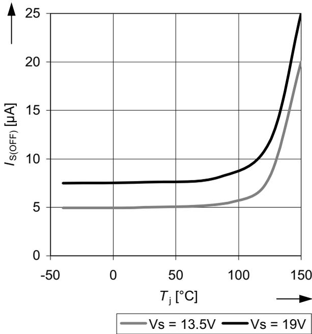
**Figure 25** Typical standby current  $I_{S(OFF)}$  as a function of the junction temperature  $T_j$
