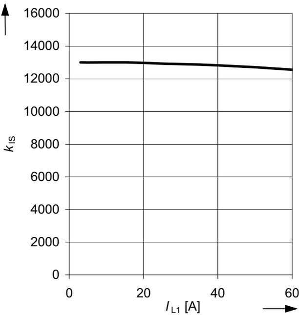
**Figure 40** Typical sense current slope  $k_{IS}$  as a function of the load current  $I_{L1}$
