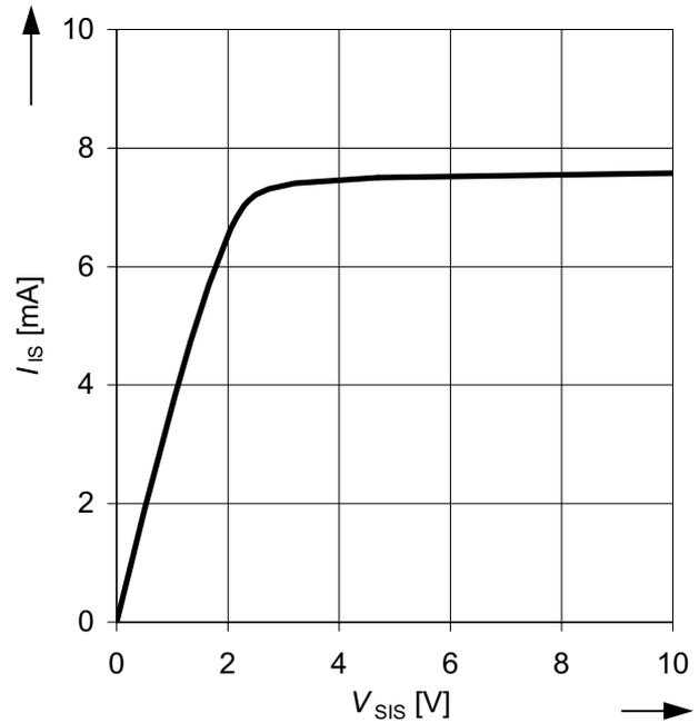
**Figure 42** Typical fault current  $I_{IS(fault)}$  at the sense output as a function of the voltage  $V_{SIS} = V_S - V_{IS}$
