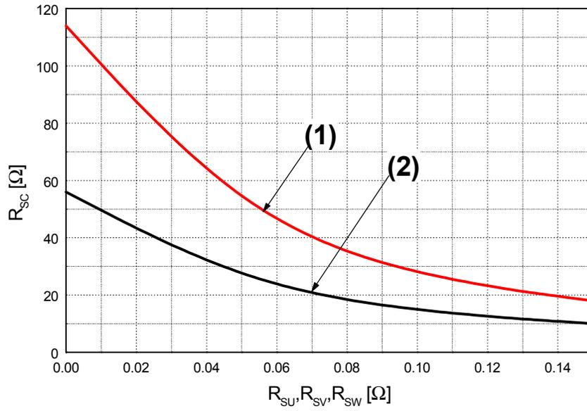
**Fig. 6.  $R_{sc}$  Variation by change of Shunt Resistors ( $R_{SU}, R_{SV}, R_{SW}$ ) for Short-Circuit Protection**
