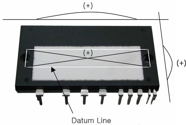
**Fig. 7. Flatness Measurement Position of The Ceramic Substrate**
